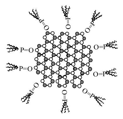
**Figure 2.** Schematic representation of a CdSe nanocrystal considered in this work. Because of the synthetic route followed to its preparation, a CdSe nanocrystal is characterized by a semiconductor core surrounded by TOPO chains anchored to its surface.
