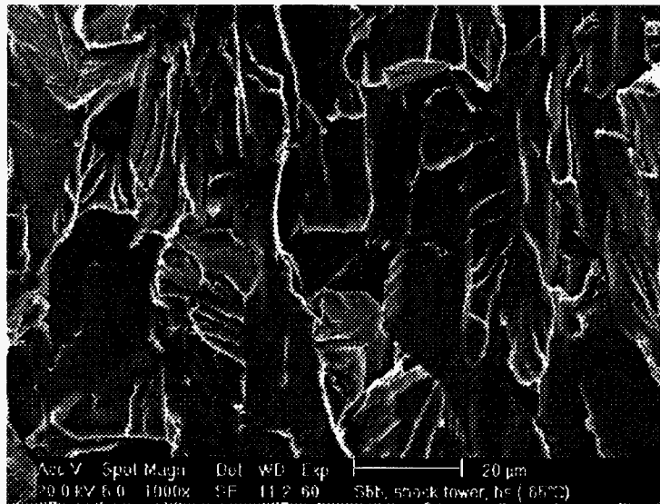
b) Fracture surface in an area with 70-80% strain, specimen fractured at -65^{\circ}\text{C}
