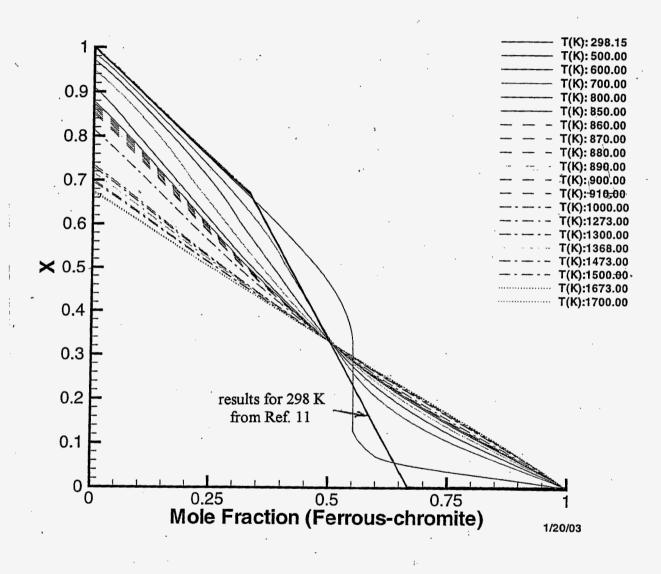
Fig. 5. Fraction of tetrahedral site  $Fe^{2+}$  ions disordered to octahedral sites in the  $Fe(Fe_{1-n}Cr_n)_2O_4$  spinel binary, accounting for configurational entropy changes due to electron hopping and coupling caused by alignment of magnetic moments of tetrahedral site  $Fe^{3+}$  ions vs. those of octahedral site  $Fe^{3+}$  and  $Fe^{2+}$  ions.
