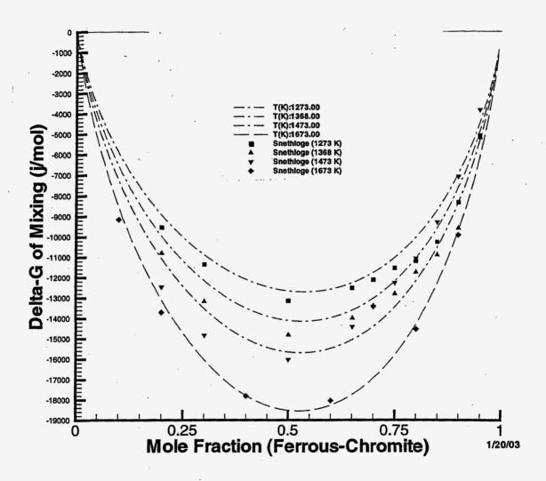
Fig. 6a. Comparison of measured and predicted free energies of mixing in the Fe(Fe<sub>1-n</sub>Cr<sub>n</sub>)<sub>2</sub>O<sub>4</sub> spinel binary. Data taken from Snethlage and Schröcke ( $\Box$  1273 K,  $\triangle$  1368 K and  $\nabla$  1473 K) and Petric and Jacob ( $\Diamond$  1673 K). W = 6500 J mol<sup>-1</sup>;  $\alpha$ ,  $\beta$ ,  $\gamma$  and  $\sigma_{el}$  obtained by regression of magnetite disordering data as discussed in text.
