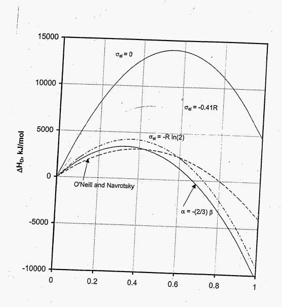
Fig. 4. Effect of  $\sigma_{el}$  constraint on enthalpies of disordering for magnetite,  $\Delta H_D$ .
