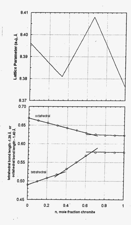
Fig. 2. M-O bond lengths inferred from spinel structure, lattice parameter and indicated cation distribution. Lattice parameter measurements shown in (a) are taken from Ref. 12.
