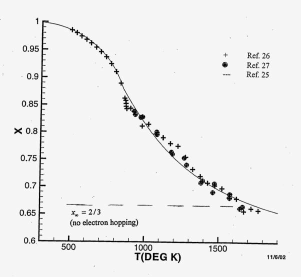
Fig. 3. Comparison of measured and fitted cation disordering parameter, x, in Fe<sub>3</sub>O<sub>4</sub>. Magnetite melts at 1870 K.
