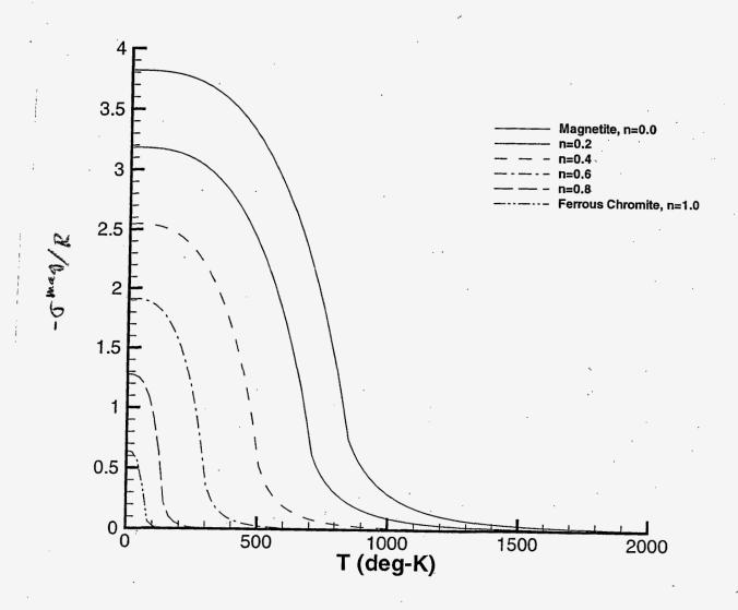
Fig. 1. Magnetic ordering contribution to entropy,  $\sigma^{\text{mag}}$ , in the Fe(Fe<sub>1-n</sub>Cr<sub>n</sub>)<sub>2</sub>O<sub>4</sub> spinel binary per Inden model.
