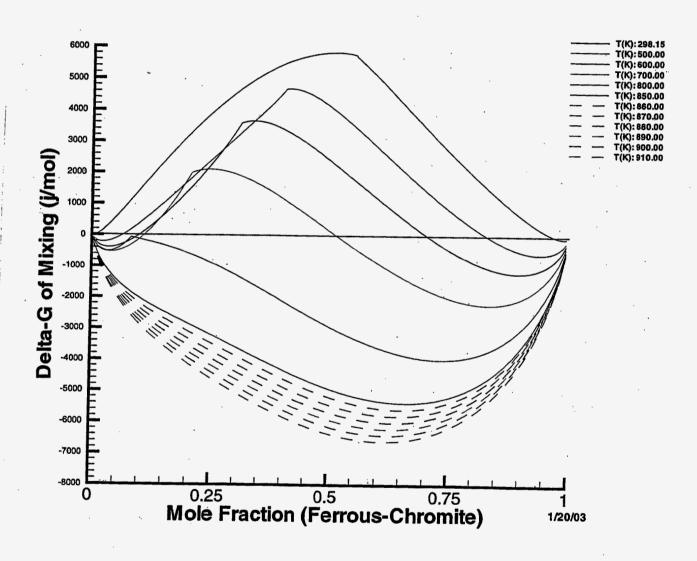
Fig. 6b. Predicted  $\Delta G_{mix}$  in  $Fe(Fe_{1-n}Cr_n)_2O_4$  spinel binary at temperatures below 1000 K. The discontinuity in slope of each  $\Delta G_{mix}$  curve below 800 K is an artifact of the Inden model and does not affect the solvus calculation, since it occurs in the two-phase region.
