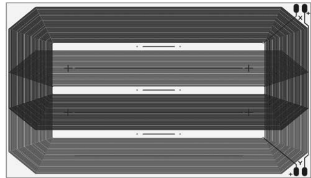
Figure 10 Kapton film flexible board of compensation coils. Coils on opposite sides (shown in red and blue) provide magnetic fields in two directions.
