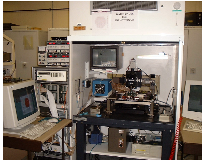
Fig. 2 A test system employed at Rutherford Appleton Laboratory. The system components are the VME board in a crate, the enclosed box on the left of the probe station housing the pin driver and connector boards, and the probe card in the probe station.
