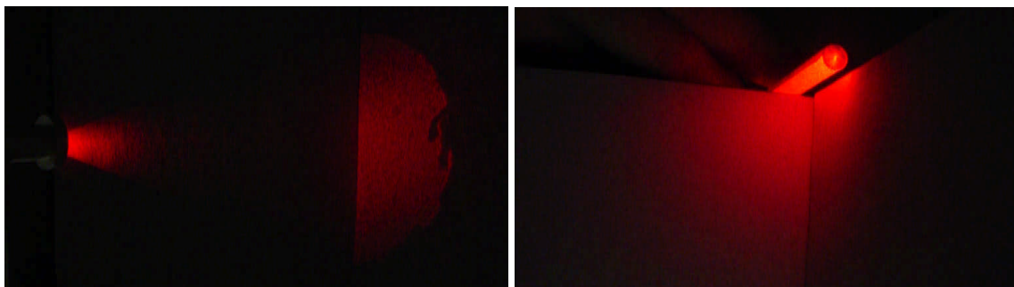
Fig. 37. Downlight (left) and waveguide (right) beam distributions
