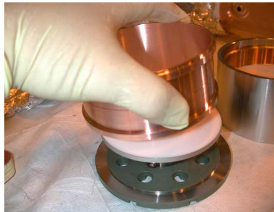
Figure 2: Ceramic brazing technique.
