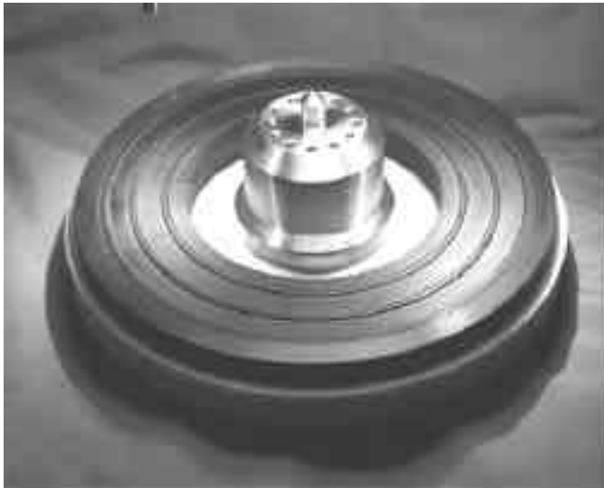
Fig. 1. Magnet assembly for an HTS bearing, shown here installed on a bearing test rotor.
