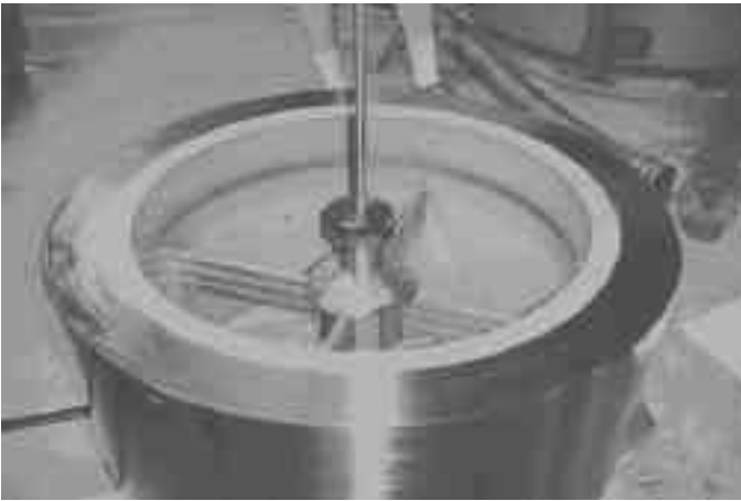
Fig. 5. Rotor for a 10-kWh flywheel after quill test at 14,000 rpm.
