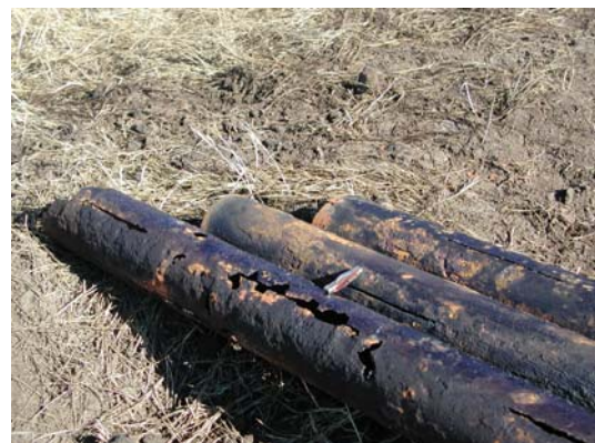
Figure 3. Liner removed from the CO2 Project #16 well in January in preparation for drilling deeper to the LKC C interval.
