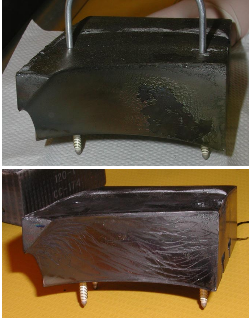
Fig. 1 TFTR tile KB3 The curved surface of the diagnostic penetration is shown (i) with the codeposit and (ii) after the codeposit was mechanically removed.
