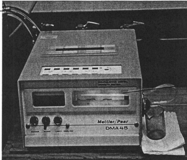
FIGURE 3.1 The Anton-Paar Digital Density Meter.
