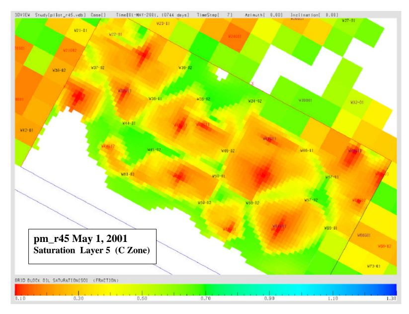
Figure 10. Original pilot model-predicted oil saturation for layer 5 (top of C Sand) at current time.
