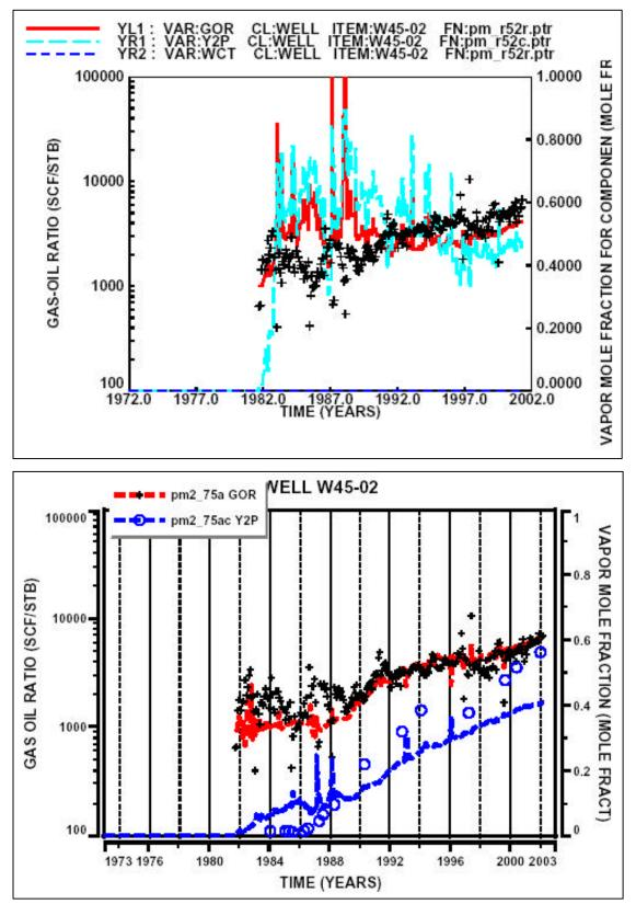
Figure 6. Simulation history match plots for EBU 45-2. The upper plot is the match from the original pilot model; the lower plot is from the current model. "Y2P" is the nitrogen content of produced gas. Symbols are field data; lines are model data.
