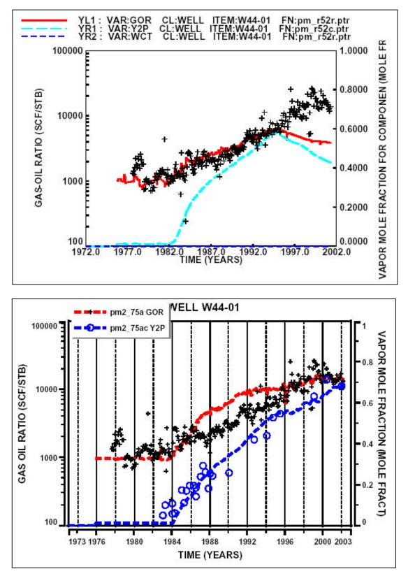
Figure 5. Simulation history match plots for EBU 44-1. The upper plot is the match from the original pilot model; the lower plot is from the current model. "Y2P" is the nitrogen content of produced gas. Symbols are field data; lines are model data.
