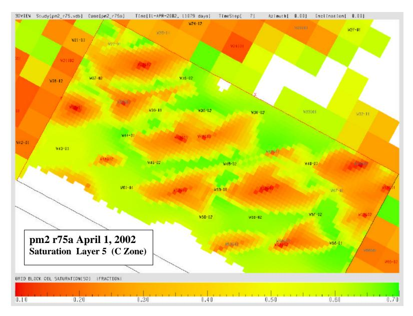
Figure 11. Current pilot model-predicted oil saturation for layer 5 (top of C Sand) at current time.
