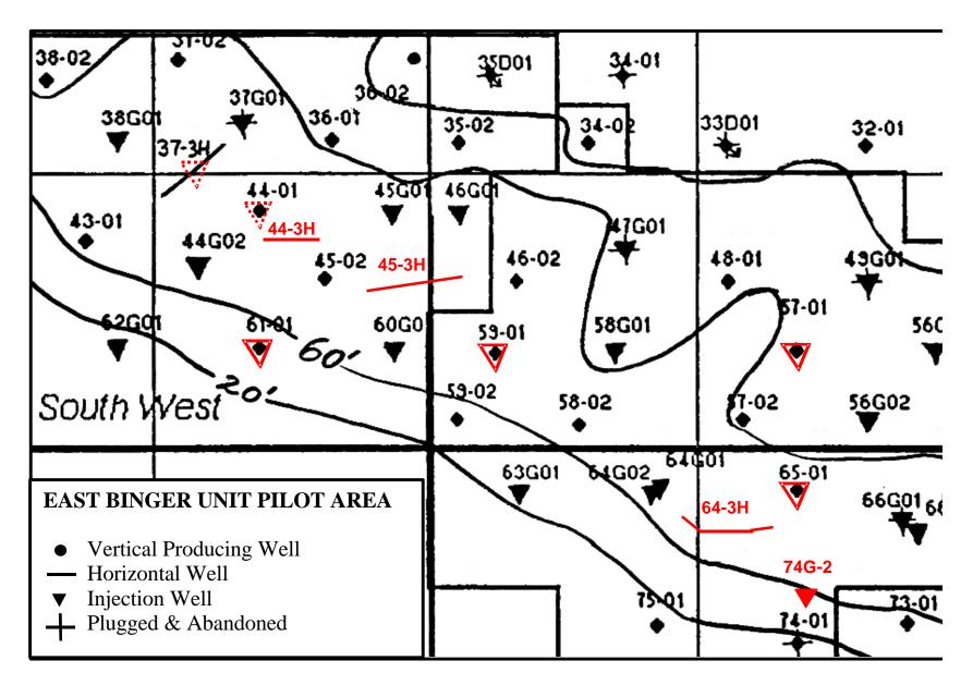
Figure 2. Fieldwork planned for the pilot - shown in red. Either 37-3H or 44-1 will be converted to injection.
