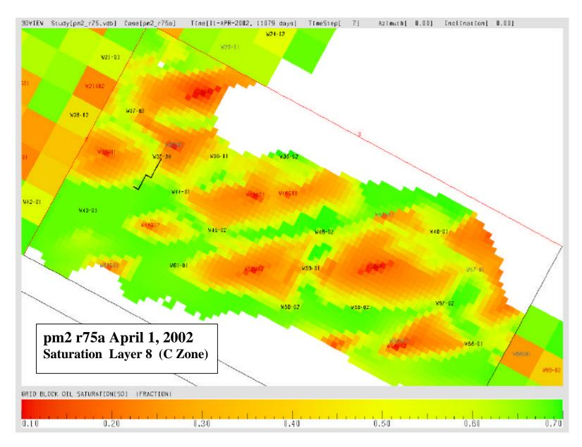
Figure 9. Current pilot model-predicted oil saturation for layer 8 (middle of C Sand) at current time.
