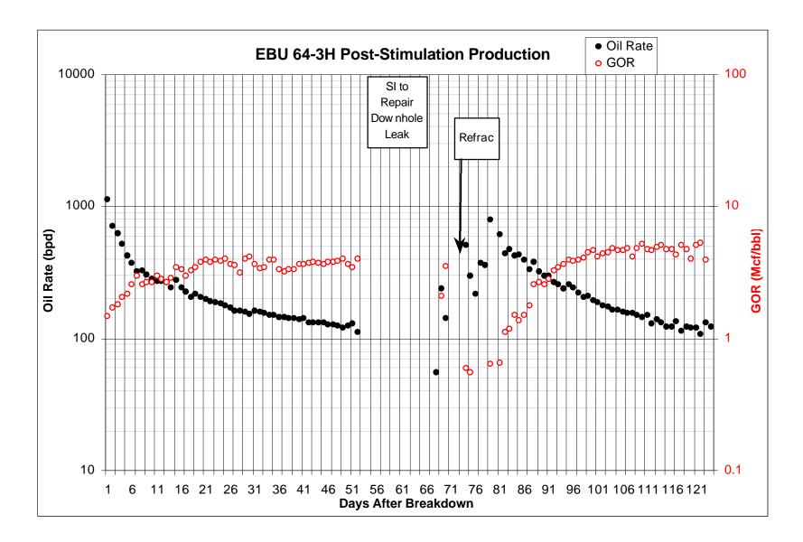
Figure 3. Post-stimulation production data for horizontal well EBU 64-3H. The breakdown treatment was pumped in early September 2002.
