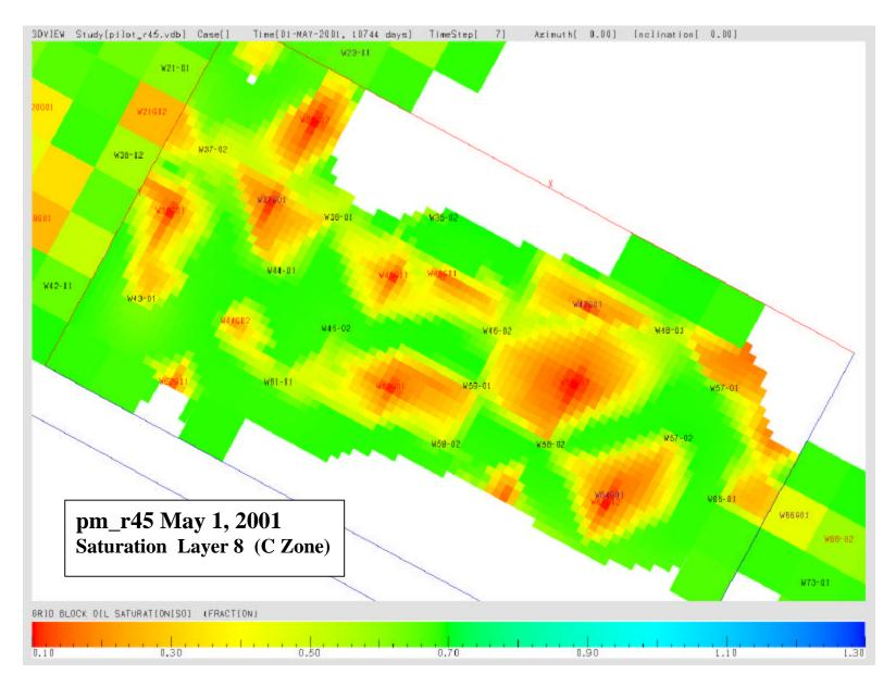
Figure 8. Original pilot model-predicted oil saturation for layer 8 (middle of C Sand) at current time.
