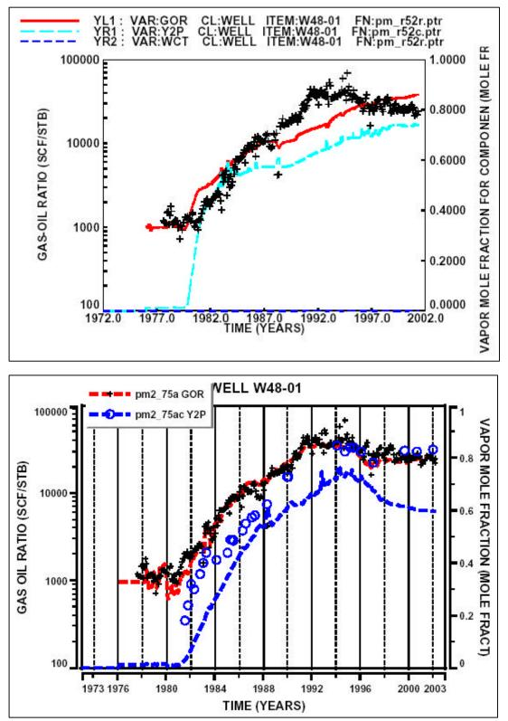
Figure 7. Simulation history match plots for EBU 48-1. The upper plot is the match from the original pilot model; the lower plot is from the current model. "Y2P" is the nitrogen content of produced gas. Symbols are field data; lines are model data.
