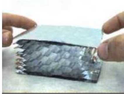
Figure 1. Example of multilayered GFP (Photo: Goudey, LBNL)
