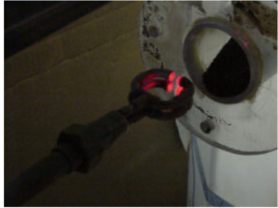
Dual optical particle counter probe removed from the column with the light sources illuminated
