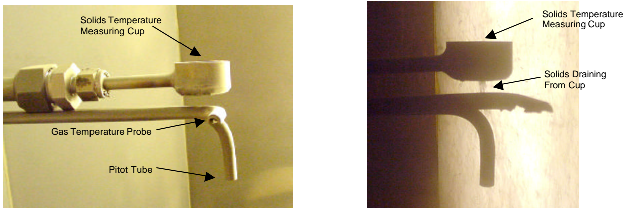
Figure 3.1-12: Solids Temperature Probe
