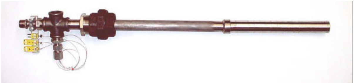
Figure 5.5-1: Assembled Materials Test Probe
