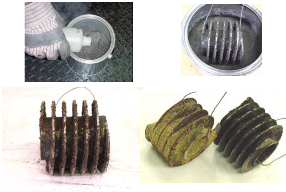
Figure 3.2-6: Tube Leak Simulation with CMB Ash
