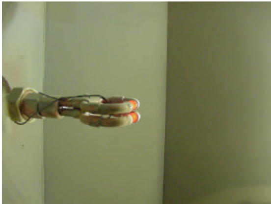
Dual optical particle counter probe installed in the test column
