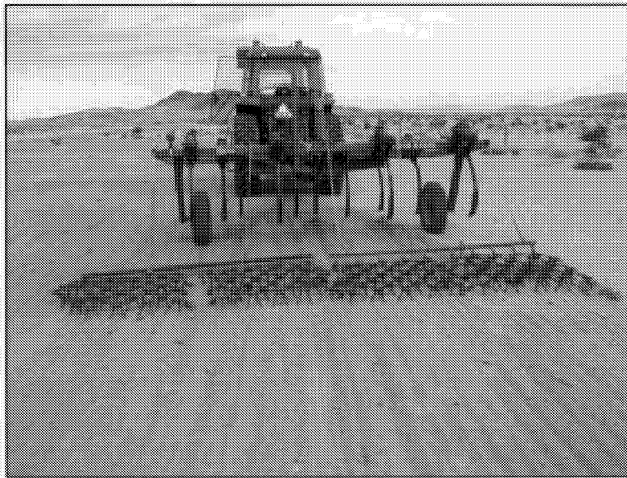
Figure 3-9. Chisel-tooth plow followed by a drag harrow used to reduce compaction and roughen the upper 10-15 cm (4-6 in) of the soil.
