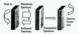
Photon Radiator Spectral Control Device TPV Diodes
