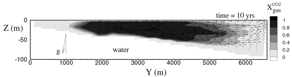
Figure 7. CO<sub>2</sub> mass fraction in the gas and gas velocity vectors after 10 years of CO<sub>2</sub> injection into a heterogeneous reservoir.
