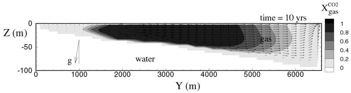
Figure 5. CO<sub>2</sub> gas mass fraction and gas velocity vectors after 10 years of CO<sub>2</sub> injection.
