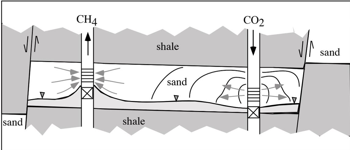
Figure 4. Cross section schematic of CO<sub>2</sub> injection and enhanced production of CH<sub>4</sub>.
