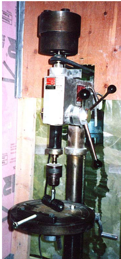
Fig. 49. Rotating-cutter drill press for abrasion resistance test
