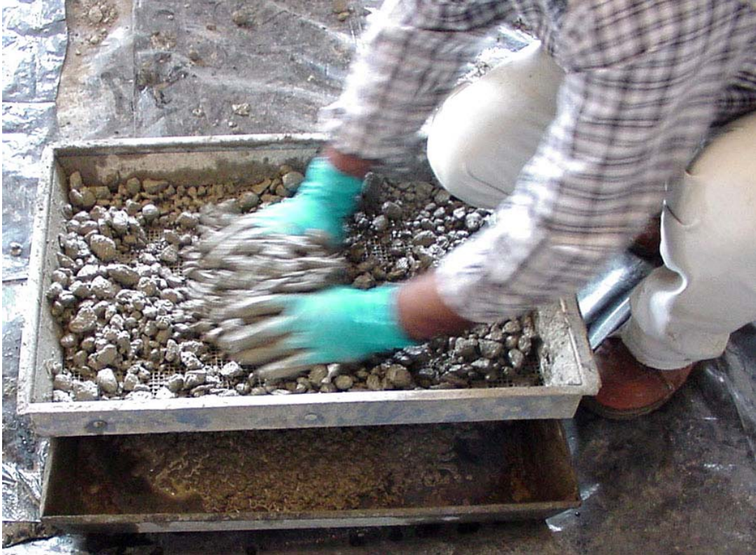
Fig. 35. Wet-sieving of concrete to obtain mortar for time of setting test
