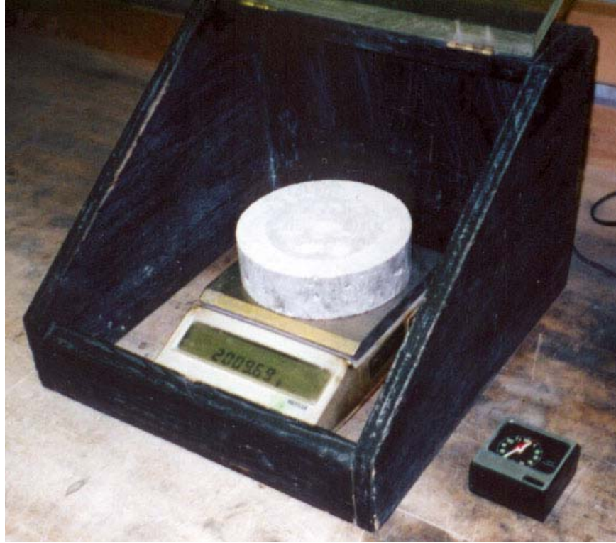
Fig. 52. Determination of mass loss due to abrasion
