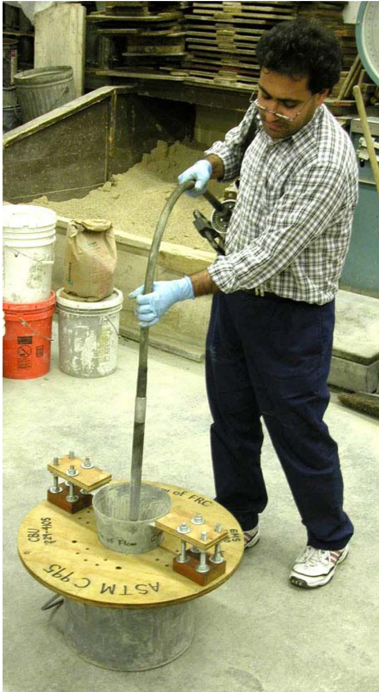
Fig. 34. Determination of time of flow of concrete (not actual testing)
