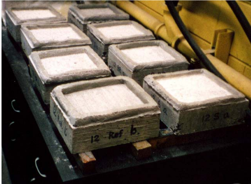
Fig. 58. Curing of salt-scaling specimens in air following 14 days of moist-curing
