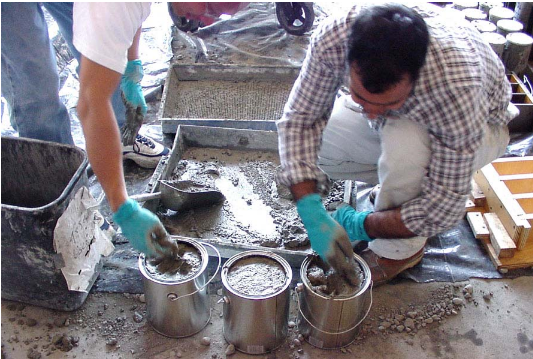
Fig. 36. Mortar samples in cans for time of setting test
