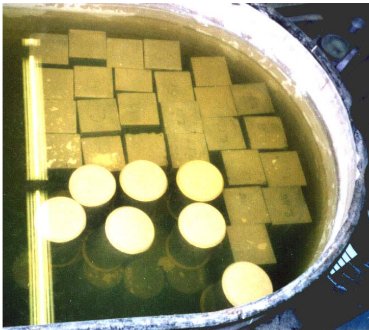
Fig. 29. Curing of specimens in lime saturated water
