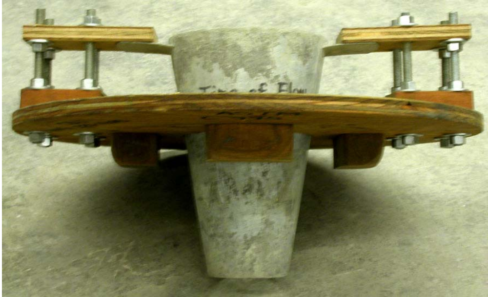
Fig. 32. Inverted slump cone for time of flow test (viewed from side)
