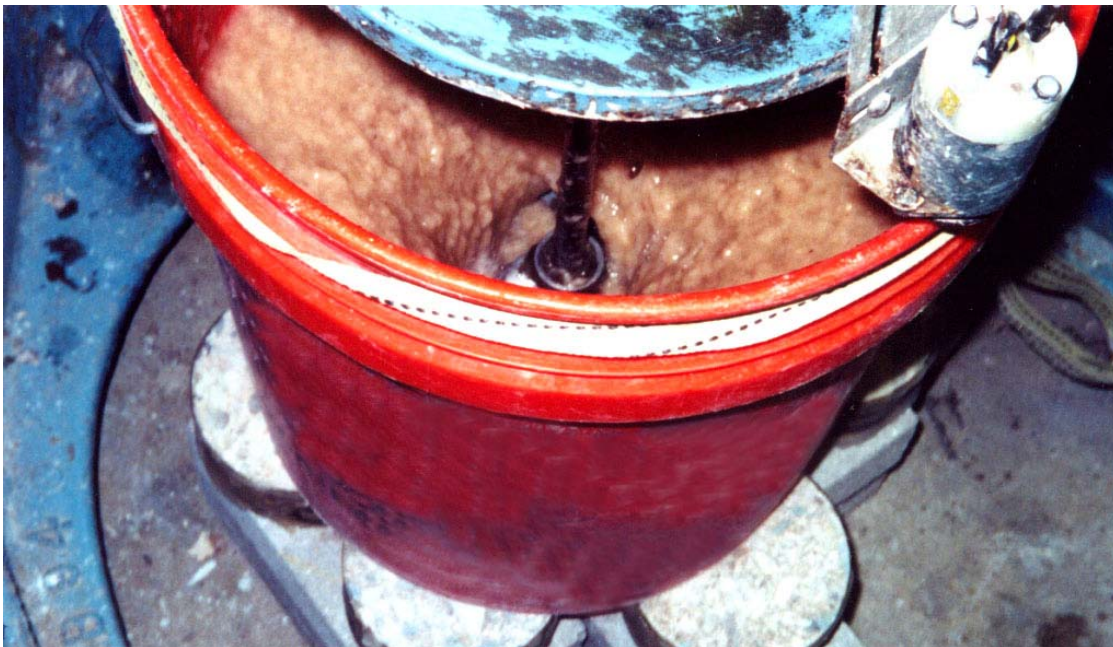
Fig. 27. Residual BR being repulped in water
