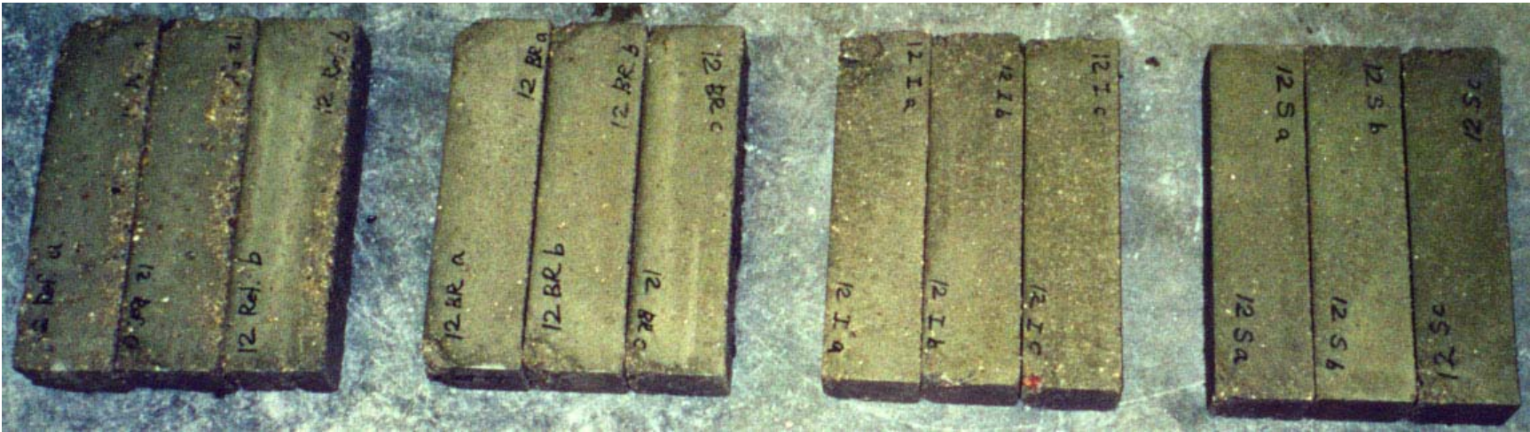
Fig. 118. Specimens after 300 cycles of freezing and thawing (Series 12)
