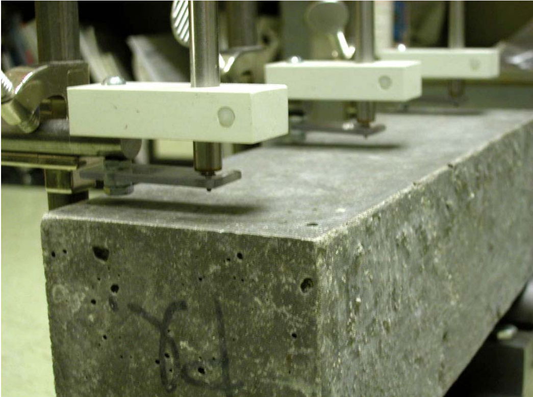
Fig. 136. LVDTs with their tips held back for setting the beam on supports
