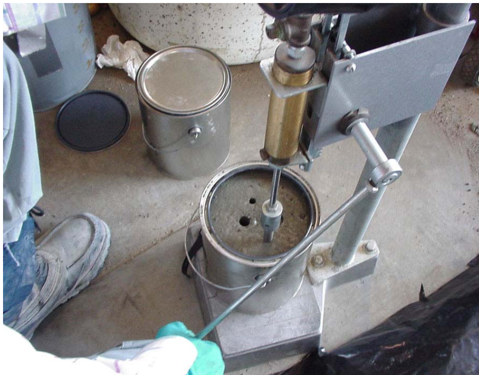
Fig. 38. Determination of penetration resistance (time of setting test)
