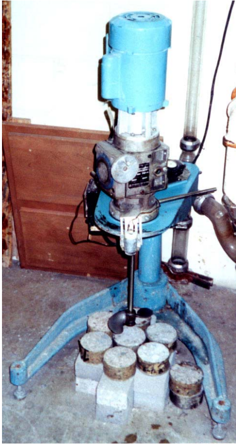
Fig. 26. High-speed motor with a rotor for “repulping” residuals
