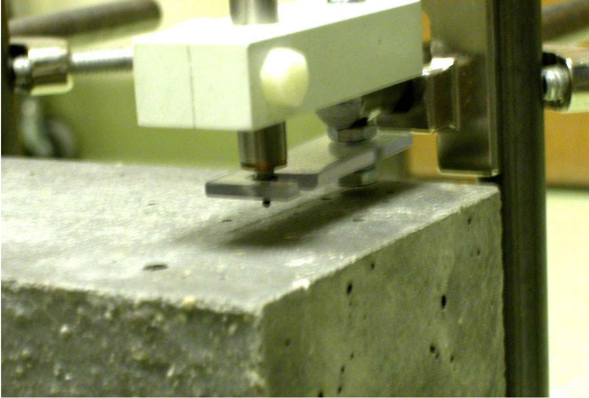
Fig. 138. Stopper holding back the tip of LVDT
