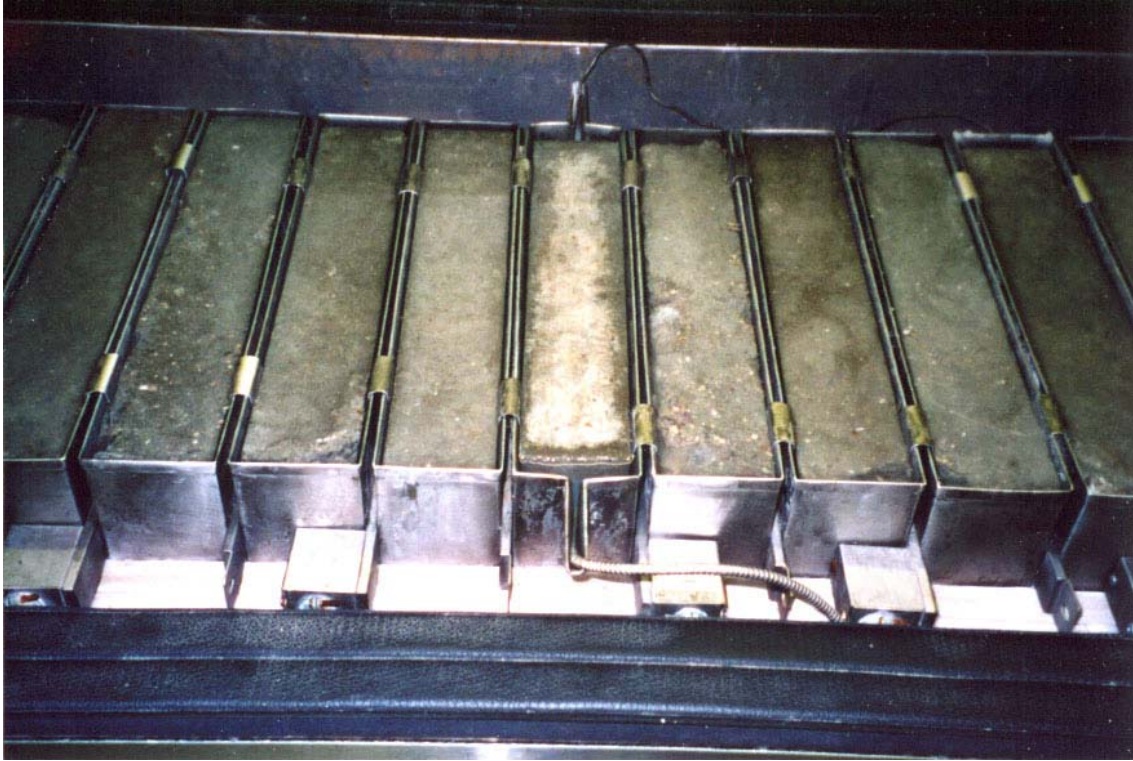
Fig. 54. Temperature control specimen (middle) with thermocouples
