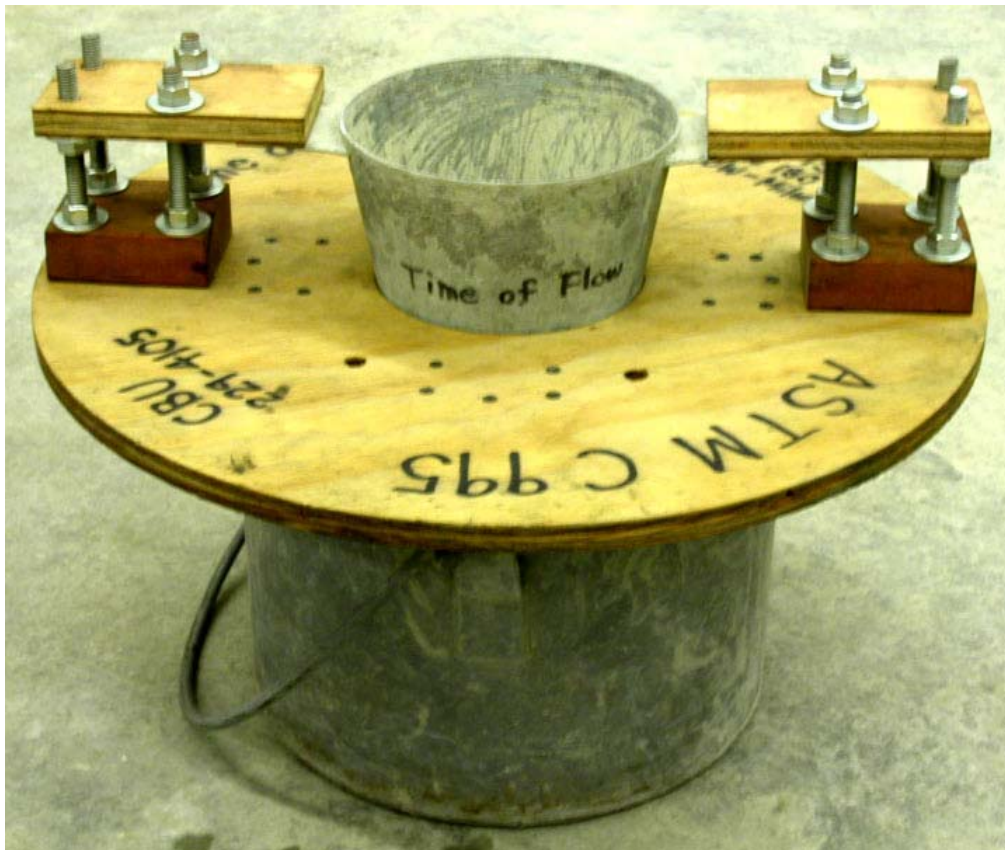
Fig. 33. Inverted slump cone set on top of ASTM C 29 one-ft 3 bucket (There is a 4" clearance between the small end of the cone and the bottom of the bucket. Two vent holes are visible on plywood disk.)
