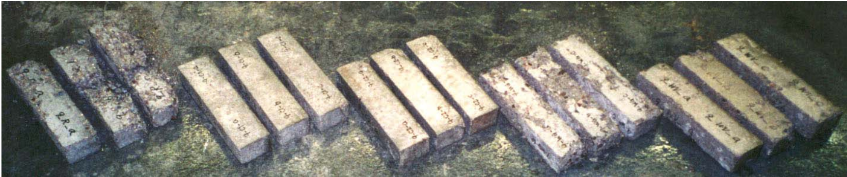
Fig. 117. Specimens after 300 cycles of freezing and thawing (Series 9)
