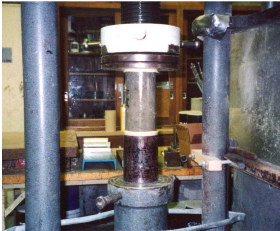
Fig. 40. Concrete cylinder under compressive load
