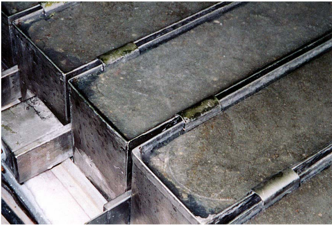
Fig. 55. Freezing-and-thawing specimens frozen at the end of freezing phase
