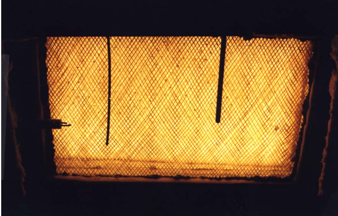
Figure 22. Photograph of holmium coated CFCC burner at 15,000 Btu/hr firing rate.
