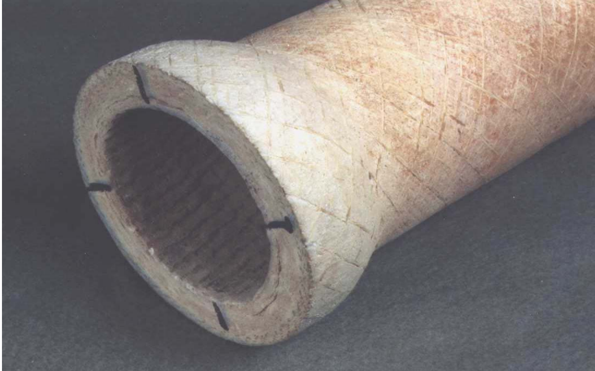
Figure 4. Net shape flange produced by vacuum winding.
