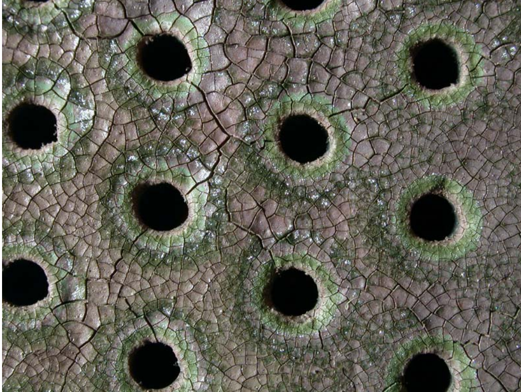
Figure 28. 8X macrophoto of "black body" coated burner block following the IPST testing.
