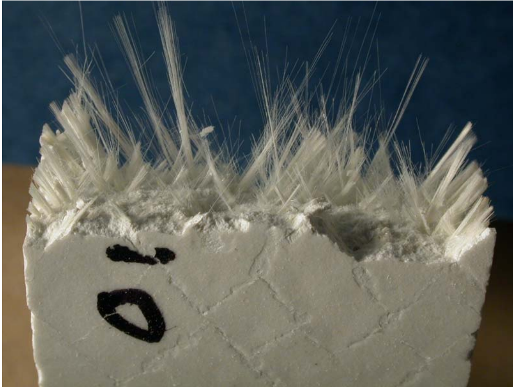
Figure 13. Fracture surface of C-ring sample showing extensive fiber pull-out (7X).
