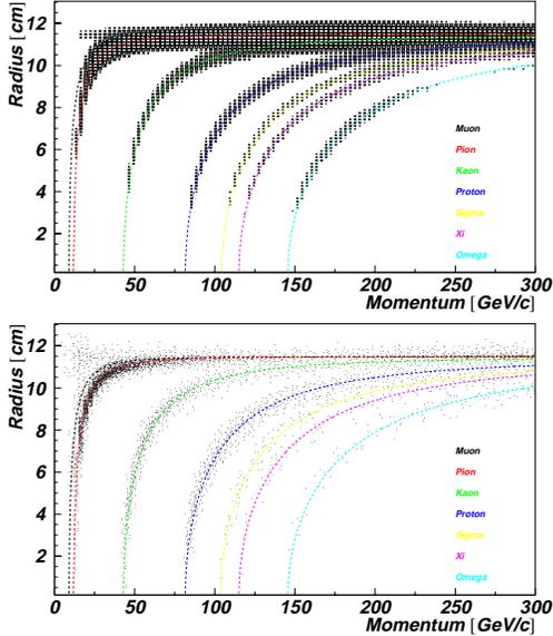
Fig. 1. Distribution of ring radii and momentum for single track events. Top:  $53 \cdot 10^6$  negative tracks. Bottom: 180000 positive tracks. The lines show the expected for ring radii for  $\mu^\pm$ ,  $\pi^\pm$ ,  $K^\pm$ ,  $p^\pm$ ,  $\Sigma^\pm$ ,  $\Xi^\pm$ , and  $\Omega^\pm$ .
