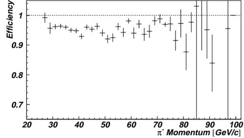
Fig. 3. Identification efficiency for  $\pi^-$  as function of momentum.
