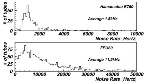
Fig. 2. Distribution of noise rates (conservative estimate) for the two types of phototubes used in the detector.
