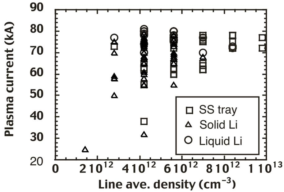
Figure 2. Plasma current – line averaged density operating space for CDX-U with an empty stainless steel tray limiter, a solid lithium fill, and a liquid lithium fill. The horizontal grouping of the density data is due to a binning algorithm.
