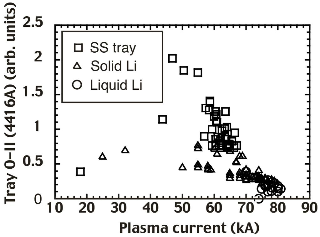
Figure 3. Oxygen II emission at the surface of the tray, for discharges limited by the empty tray, a solid lithium fill, and a liquid lithium fill.
