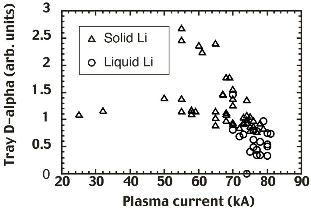
Figure 4.  $D_{\alpha}$  emission at the lithium filled tray, for solid and liquid lithium limited discharges.
