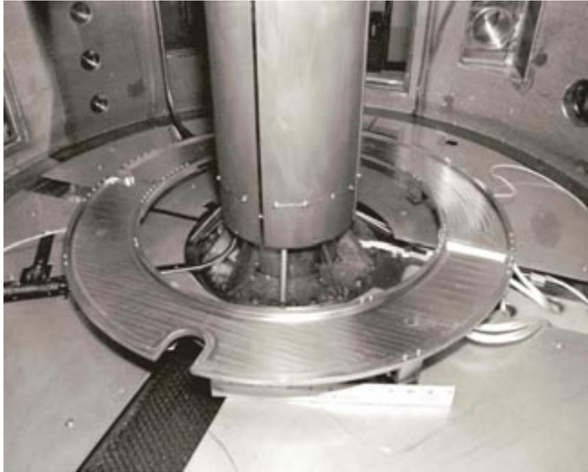
Figure 1. Photograph of the interior of CDX-U following installation of the tray limiter.
