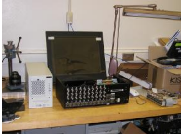
Figure 1. Front View of Data Acquisition System (DAS)
