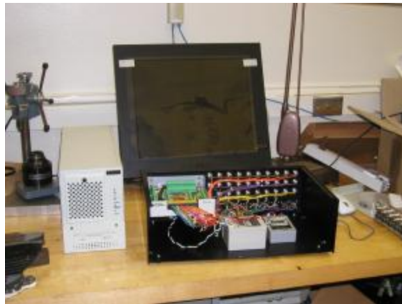
Figure 2. Rear View of Data Acquisition System (DAS)
