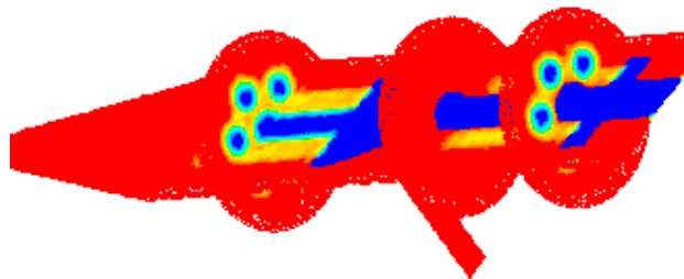
Figure 4. Contour plot for variations of the static pressure at the vessel mid-section.
