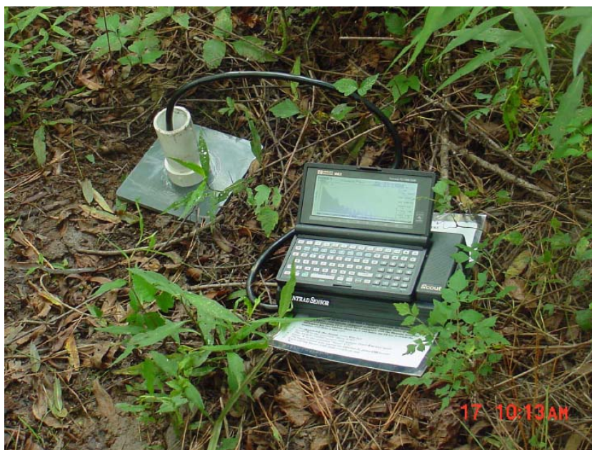
Photo 4. SCOUT Detector in Bore Hole (at bottom of hole)
