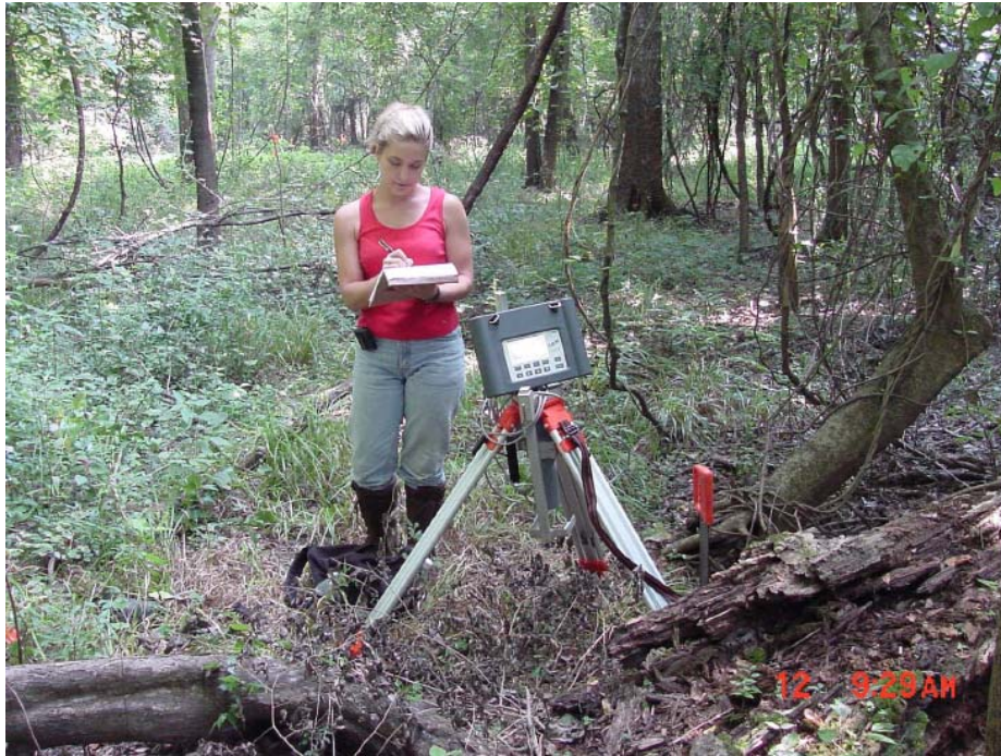
Photo 1. SAM 935 Deployed in the Field
