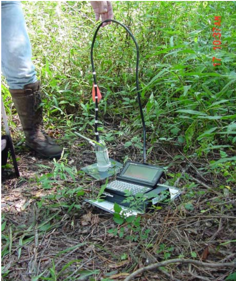
Photo 4. SCOUT Detector in Bore Hole (at bottom of hole)
