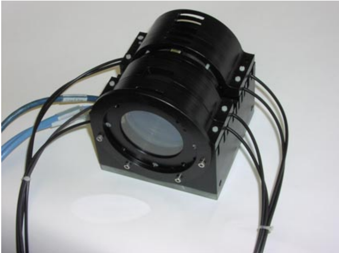
Figure 4. Photograph of 3 stage Lyot filter developed by Nova Photonics for the NSTX MSE/CIF diagnostic. Filter features electronic tuning.
