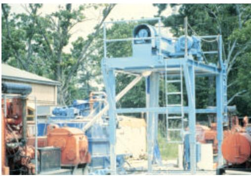
Figure 10-30. Oilfield Centrifuge Test
