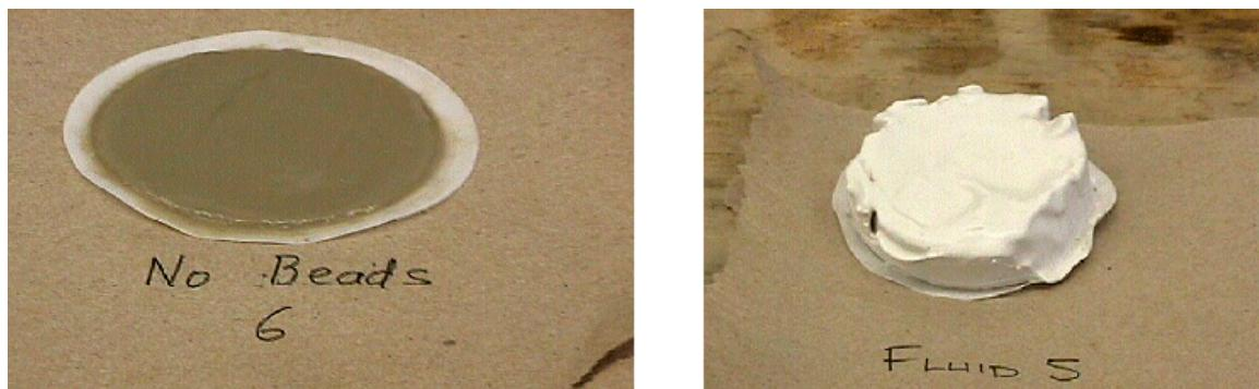
Figure 8-14. Filter-Cake Thickness Contrasted with High Fluid-Loss Filter Cake
