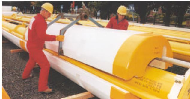
Figure 10-39. Riser Buoyancy Modules
