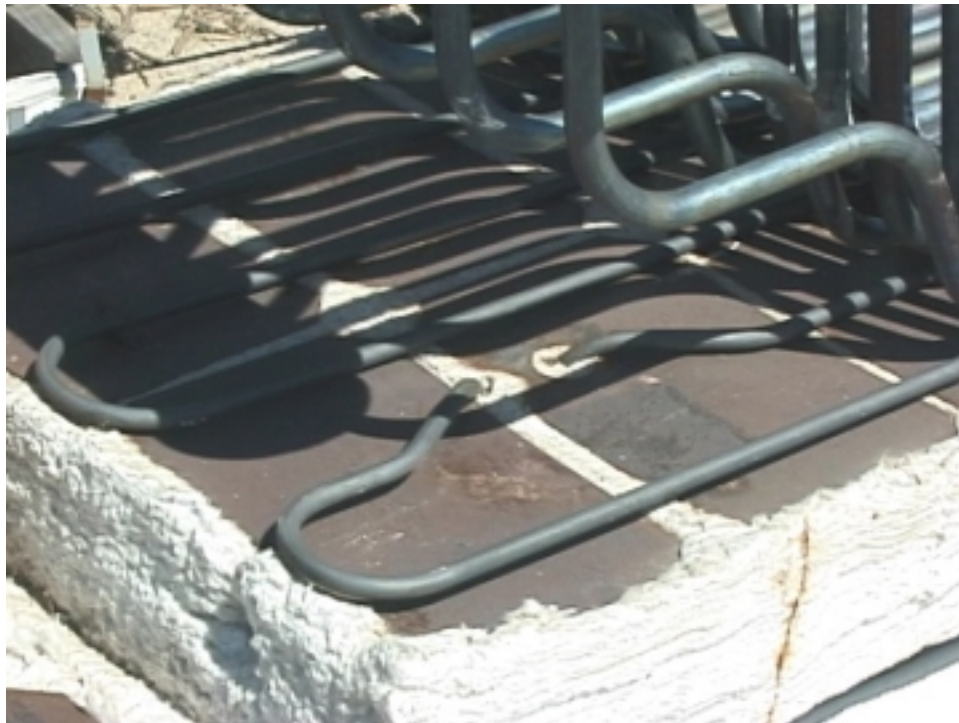
Figure A-4. Panel Electrical Heaters
