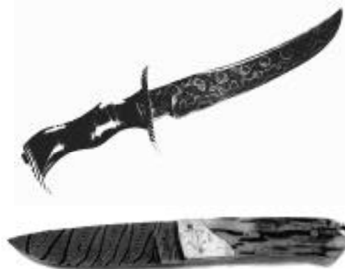
Figure 11. Welded Damascus steel knives made by American blacksmiths Bill Moran (top, courtesy of W. Moran) and Devin Thomas (bottom, after Thomas[32]).
