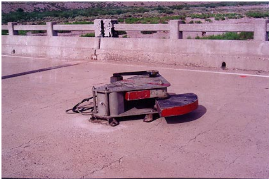
Figure 78. Eccentric mass shaker provided by the University of California at Irvine.
