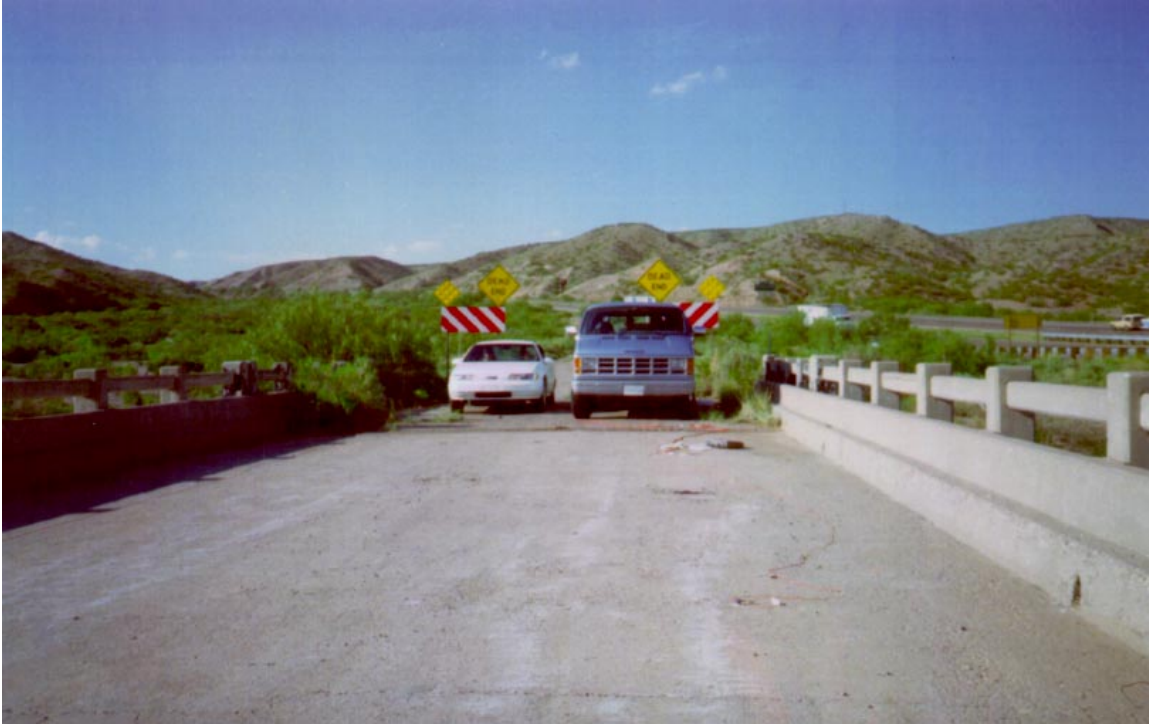
Figure 29. Ford Taurus used for ambient test two and the van containing the data acquisition equipment.
