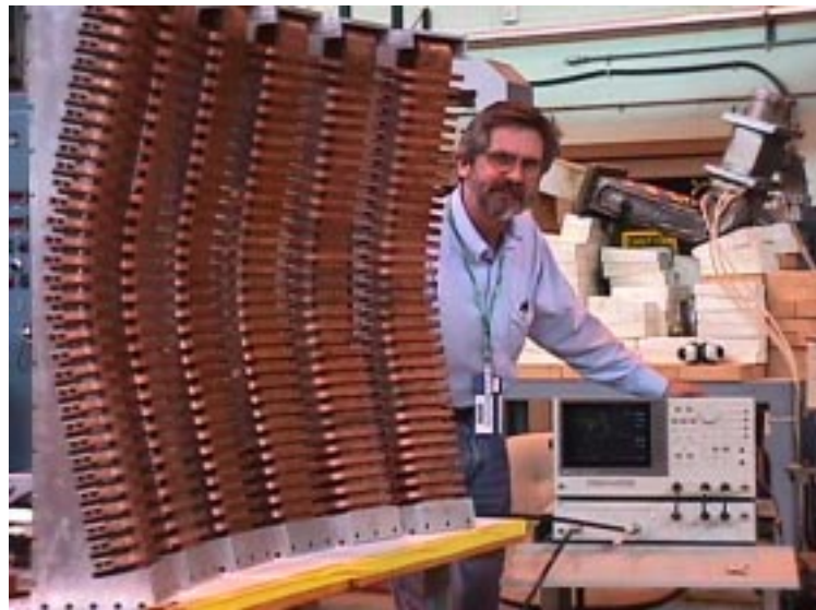
FIGURE 2. Six-element, full scale mockup of the NSTX HHFW array.
