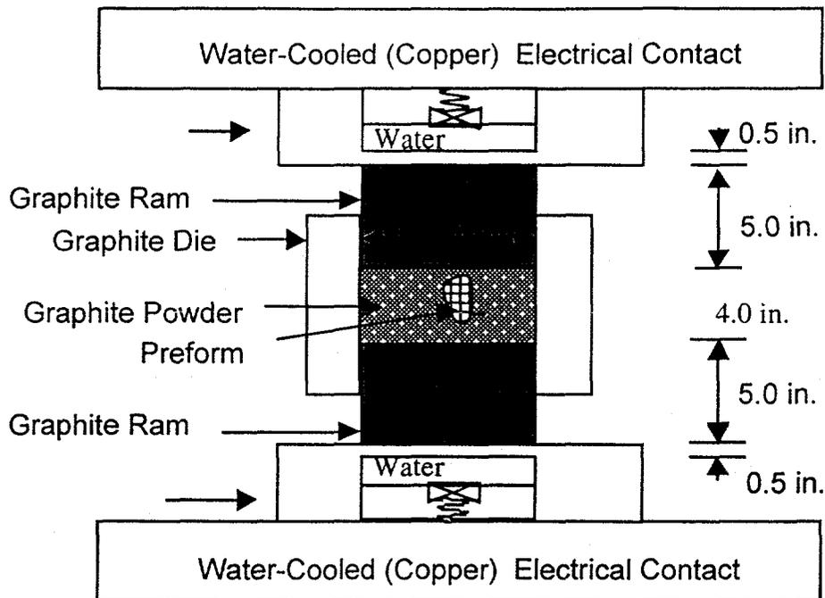
FIGURE 1. Schematic diagram of Electroconsolidation<sup>®</sup> apparatus; position of pitch-catch transducer assembly, along with typical dimensions of the die, is also shown.
