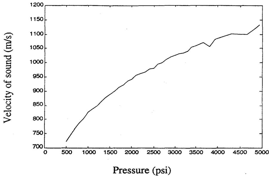
FIGURE 3. Change of velocity of sound in graphite bed with pressure at ambient temperature.
