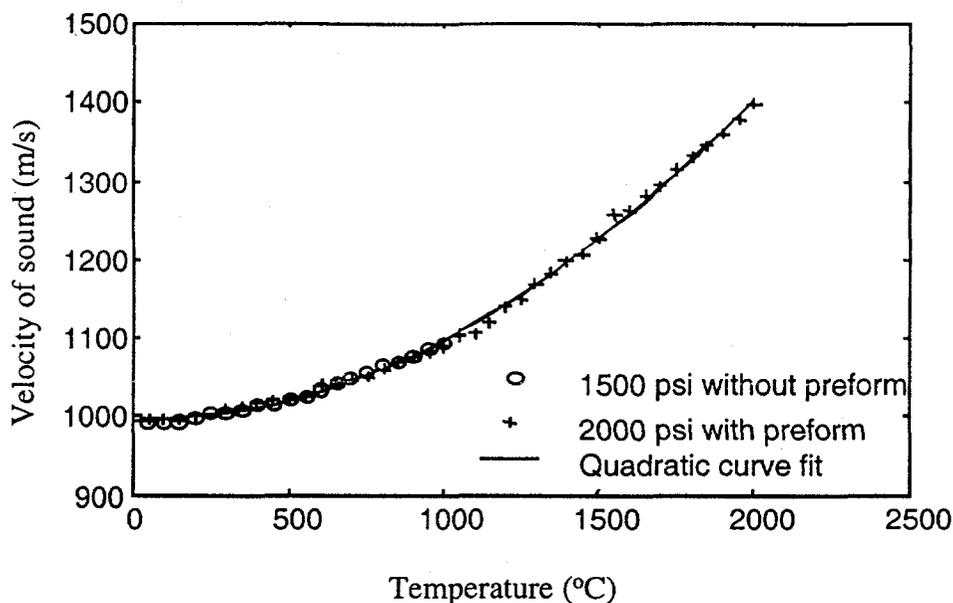
FIGURE 6. Calibration curve for a 5-inch die at 50°C/min heating rate.
