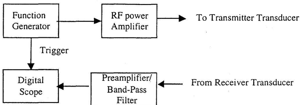
FIGURE 2. Schematic diagram of ultrasonic pitch-catch sensor electronics.
