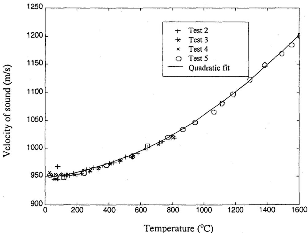
FIGURE 4. Calibration curve for a 3-inch die at 50°C/min heating rate.
