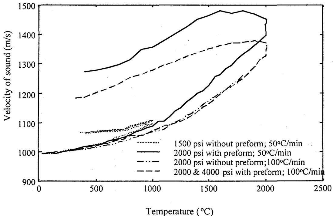
FIGURE 5. Change of ultrasonic velocity with temperature in graphite bed at fixed pressures and heating rates.
