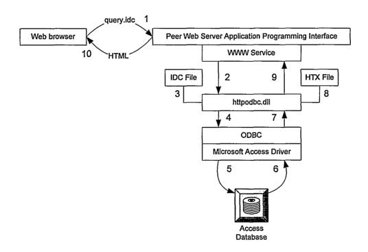
Figure 3: Web to Database Architecture
