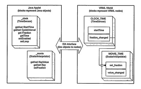
Figure 8: VRML to Java Mapping via EIA Interface
