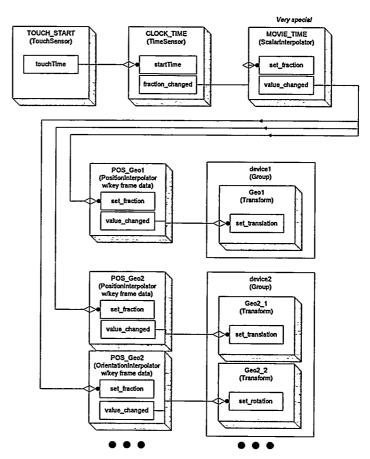
Figure 7: VRML routing required for animation control.
