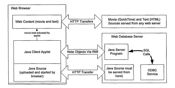
Figure 6: Network Diagram of Sandia's Digital Movie Commenting System
