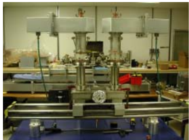
Figure 6: FPCs mounted on connecting waveguide
