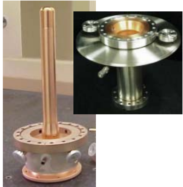
Figure 2: Window and inner conductor (a) and outer conductor (b)
