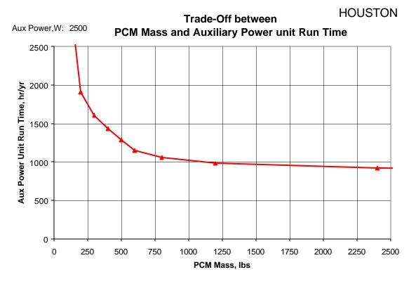
Figure 23. PCM Mass vs. Run Time (Houston)
