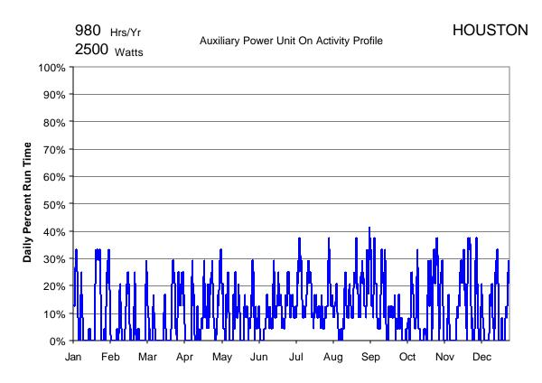
Figure 9. Auxiliary Power Use Profile (Houston-Freezer)
