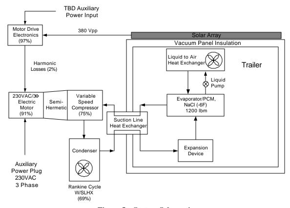
Figure 5. System Schematic
