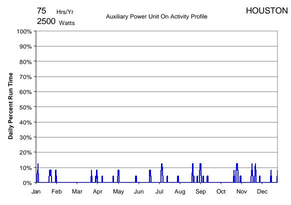
Figure 22. Auxiliary Power Use Profile
