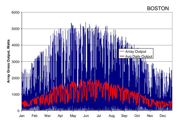
Figure 14. Array Output - Boston
