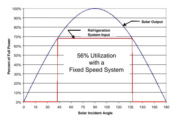
Figure 1. Fixed Speed Solar Utilization
