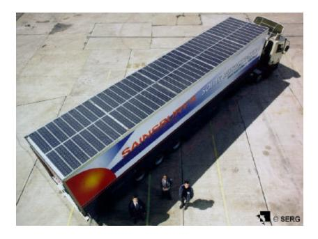
Figure 1. Solar PV Refrigerated Trailer
