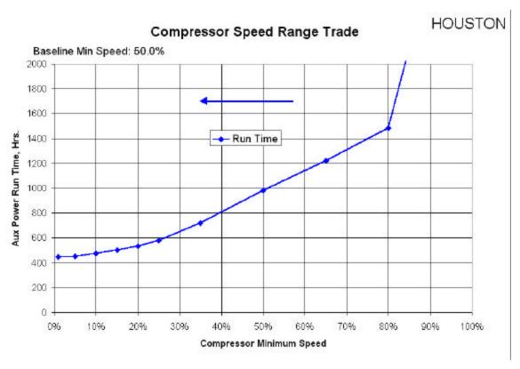
Figure 25. Compressor Speed Range vs. Run Time (Houston)
