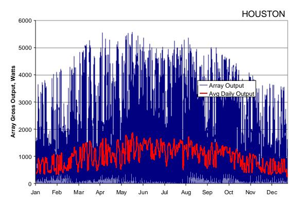
Figure 6. Solar Array Output (Houston)
