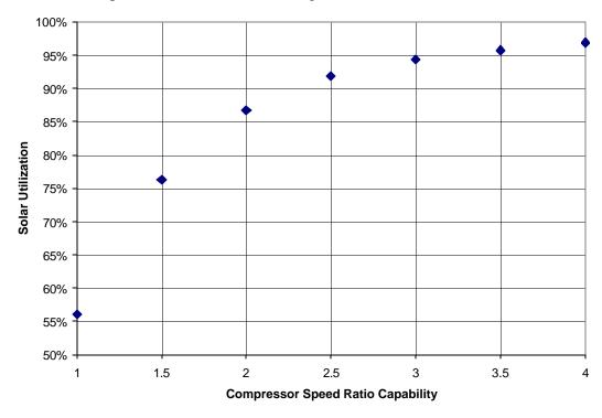
Figure 3. Solar Utilization with Different Speed Ranges
