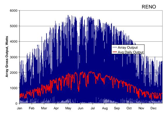
Figure 18. Array Output - Reno
