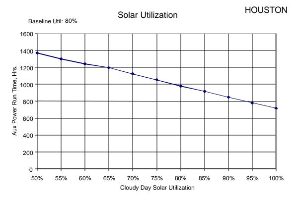
Figure 29. Solar Utilization vs. Run Time (Houston)
