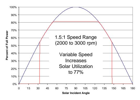
Figure 2. Solar Utilization with 1.5:1 Speed Compressor
