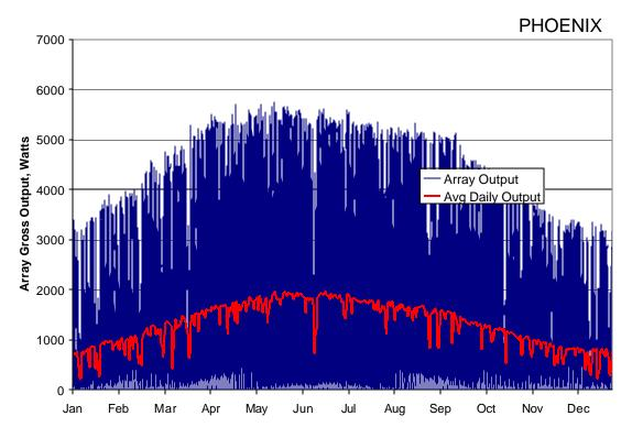
Figure 10. Array Output - Phoenix
