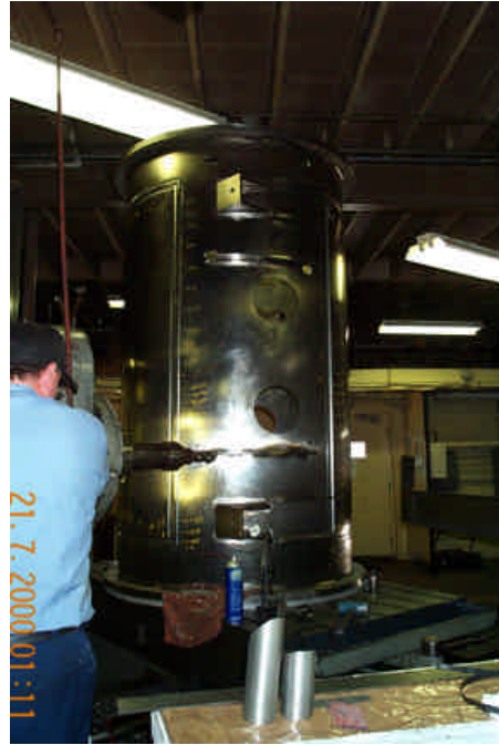
Figure 6 Milling the o-ring groove on the cryostat
