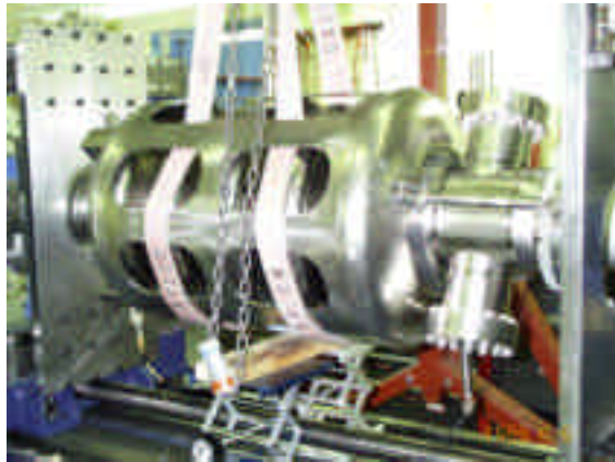
Figure 2 Cavity with inner helium vessel installed
