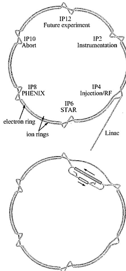
Figure 1: In the *ring-ring* scenario (TOP) electrons are stored for hours in their own ring. In the *linac-ring* scenario (BOTTOM) electrons circulate the ring once, before re-entering the superconducting Energy Recovery Linac.
