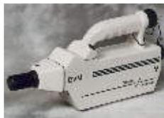
**Figure 2. Femtoscan portable GC/IMS instrument.**
