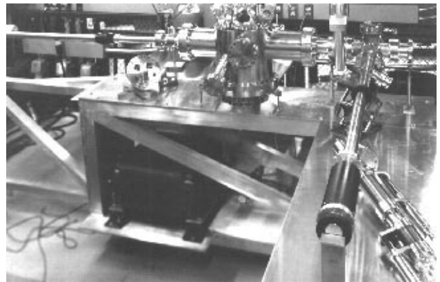
Figure 1. Cathode preparation chamber.
