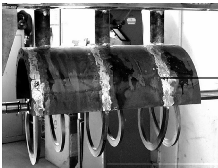
Figure 4: Resonance structure of the 5.4% power resonator directly after brazing of the arms into the half shell.
