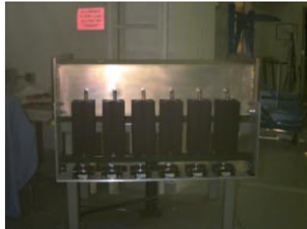
Figure 4: Photograph of LEDA 350 MHz Harmonic Filter.
