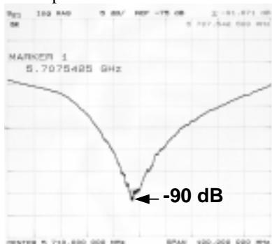
Figure 6: Frequency response of choke cavity.
