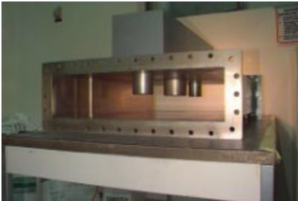
Figure 2: Photograph of 350 MHz WR2300 half-height Phase Shifter.
