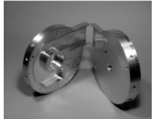
Figure 4: Machined copper parts of field symmetric double feed coupler. They will be brazed together and mounted at both ends of the structure by the electron-beam welding.
