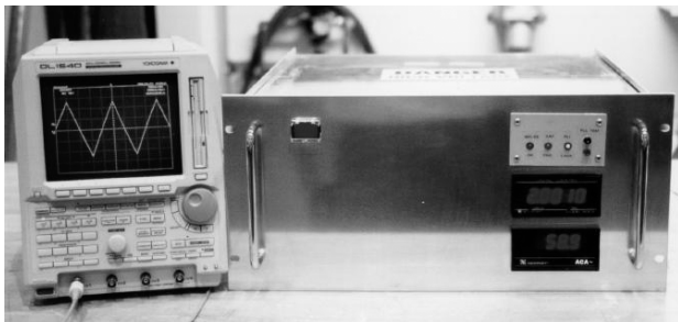
Figure 6: Modulator and test waveform (+/-100 A, 500 Hz)
