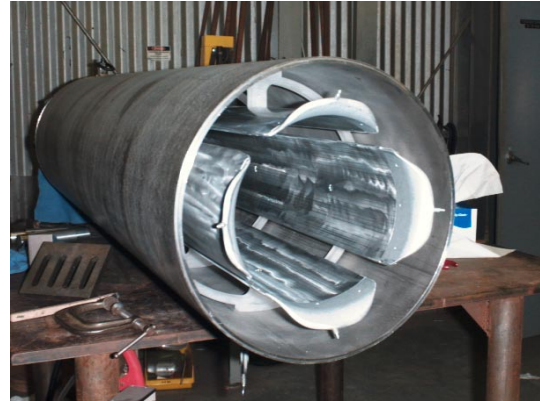
Figure 1: Photo of kicker cross-section which shows kicker plates
