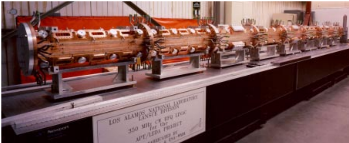
Figure 4: APT/LEDA RFQ Assembled for Pre-Installation RF Tuning
