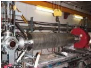
Figure 1. The quad-kicker in the Experimental Test Accelerator (ETA-II) beamline as part of the verification experiments [4]. Note the four ports on each end of the quad-kicker. These ports connect directly to the deflection plates. Two of the white pulser cables are visible in the foreground.
