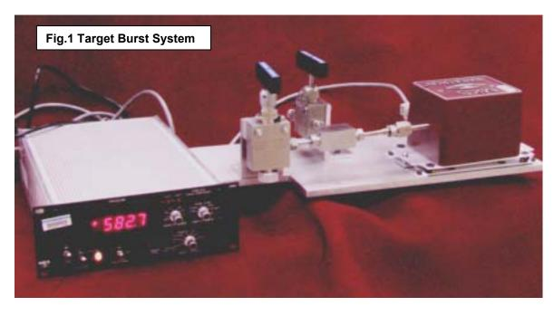
volume of 2.5cc is the limiting factor in minimizing the total internal volume. A section of the connecting tubing was stuffed with a thick walled modified AE nipple to reduce the volume 0.5cc. A measurement device with a much lower dead volume would be desirable, but the available Baratron gauge provided adequate system sensitivity for these tests. The digital read out is an MKS 270D. An Alcatel ASM110 Turbo CL leak detector was used to supply vacuum and to check for leaks in the system.
