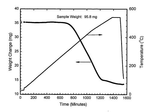
Figure A.1. Plot of Weight Change (smoothed to remove noisy signals) and Temperature Versus Time for Drying Internal Sludge ssl3, TGA Run 54
