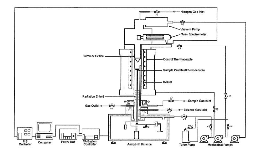
Figure 2.1. Schematic of the TGA/DSC/MS System
