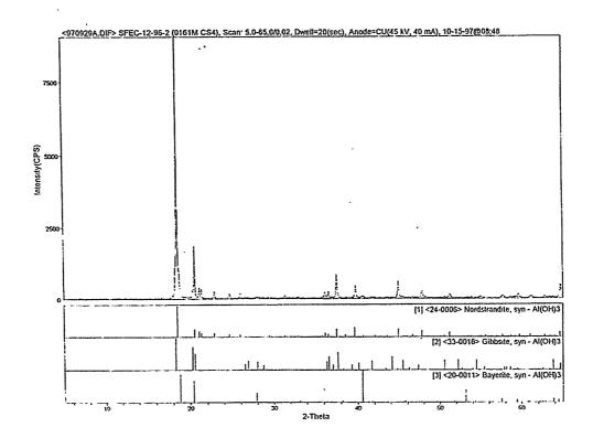
Figure A.11. Background Subtracted XRD Spectrum of SNF Surface Coating cs4. Stick figures of phases identified are included.
