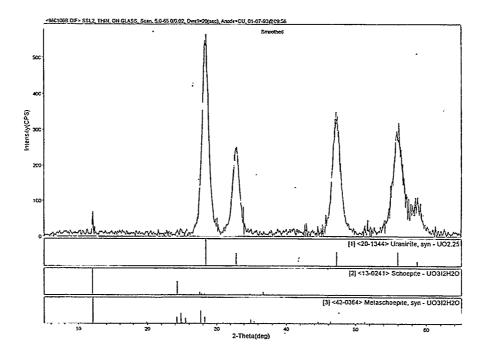
Figure A.8. Background Subtracted XRD Spectrum of SNF Internal Sludge ssl2. Stick figures of phases identified are included.
