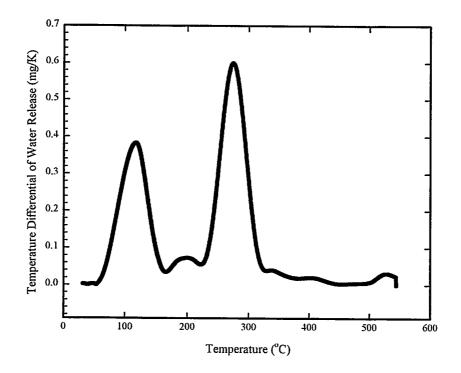
Figure A.6. Plot of the Temperature Differential of Water Release from SNF Coating Sample cs4 Derived from Figure 3.4a, TGA Run 64
