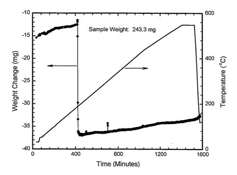
Figure A.4. Plot of Weight Change and Temperature Versus Time for Drying Internal Sludge ssl5, TGA Run 58
