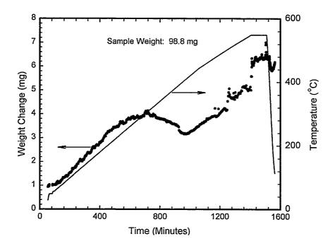
Figure A.2. Plot of Weight Change and Temperature Versus Time for Drying Internal Sludge ssl8, TGA Run 56
