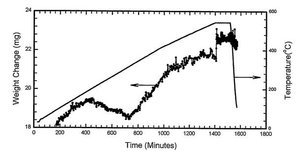
Figure A.5. Plot of Weight Change and Temperature Versus Time for Drying Internal Sludge ssl2 (2 of 3) for TGA Run 68 Showing Segment of the Run Where the Sample Lost Weight
