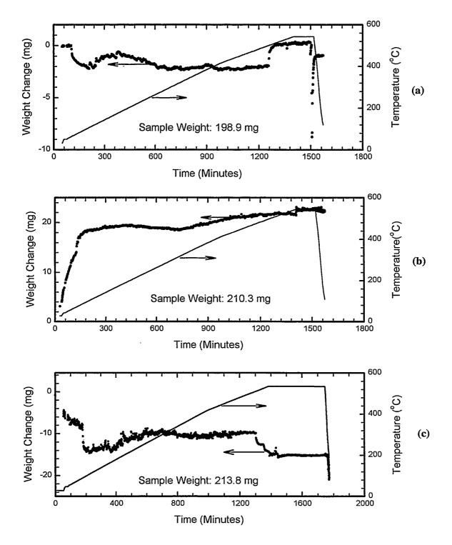
Figure 3.4. Plots of Weight Change and Temperature Versus Time for Drying the Triplicate Sample of SNF Internal Sludge ssl2; (a) 1 of 3, no prior treatment, TGA Run 67 (b) 2 of 3, prior oxidation of sample in vacuum at about 100°C, TGA Run 68 and (c) 3 of 3, prior oxidation in dry air, TGA Run 69.
