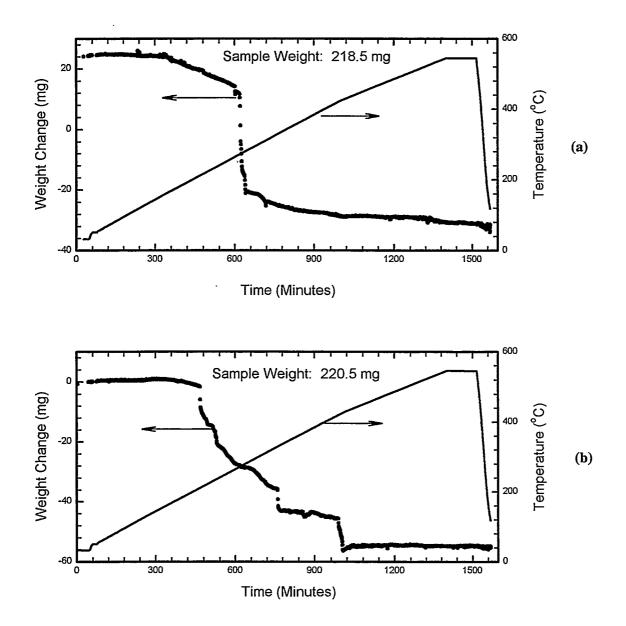
Figure 3.5. Plots of Weight Change and Temperature Versus Time for Drying SNF Coating Sample cs4 (a) First Run, TGA Run 64 and (b) Duplicate Run, TGA Run 63
