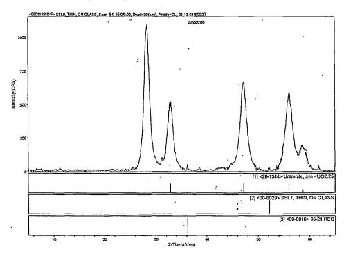
Figure A.10. Background Subtracted XRD Spectrum of SNF Internal Sludge ssl8. Stick figures of phases identified are included.
