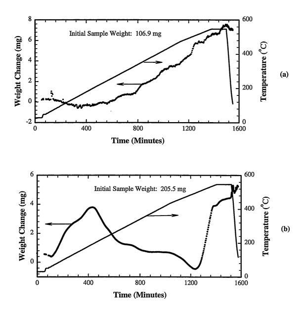
Figure 3.2. Plots of Weight Change and Temperature Versus Time for Drying Internal Sludge ssl2 (a) First Run TGA Run 53 and (b) Rerun, TGA Run 59
