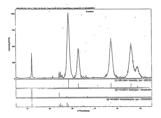
Figure A.7. Background Subtracted XRD Spectrum of SNF Internal Sludge ssl1. Stick figures of phases identified are included.
