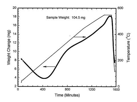
Figure A.3. Plot of Weight Change (smoothed to remove noisy signals) and Temperature Versus Time for Drying Internal Sludge ssl4, TGA Run 57
