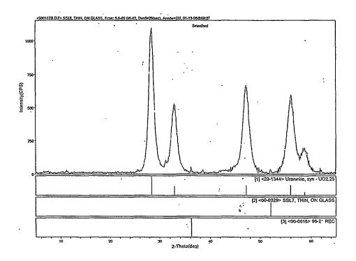
Figure A.9. Background Subtracted XRD Spectrum of SNF Internal Sludge ssl3. Stick figures of phases identified are included.
