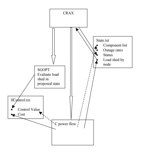
Figure 4.1. Power System Uncertainty Analysis using CRAX.
