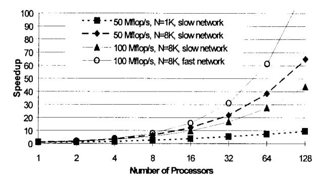
Figure 4-3 Effect of Parallel Processing on Computational Speed
