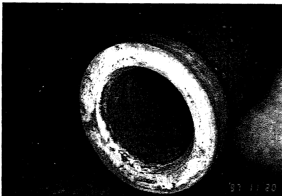
Figure 40 - Inside diameter of Karhula-exposed element before ash removal
