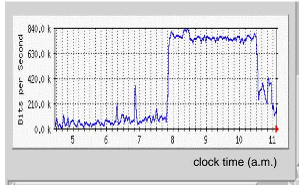
Figure 7: MRTG graph for pipechar BW usage at node 5 in Figure 5
