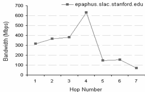
Figure 6: Pipechar test over an asymmetric path
