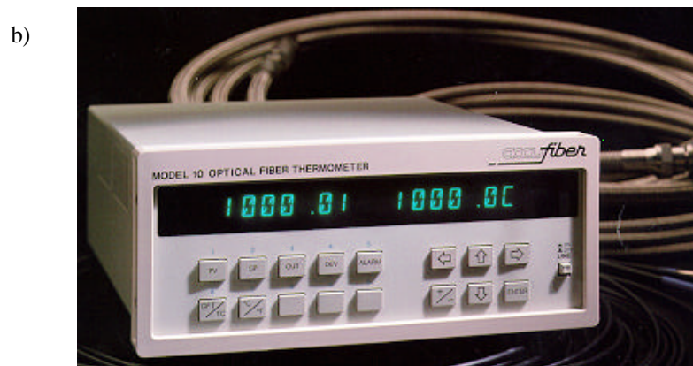
Figure 4-5 Optical fiber thermometer system: a) Pyrometer and b) Model 10 optical fiber thermometer system with a transmission cable.
