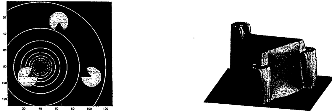
Figure 7: A strongly off center fixation point: on the left equispaced contour lines of the point-of-view surface are shown and on the right the subjective surface is visualized.
