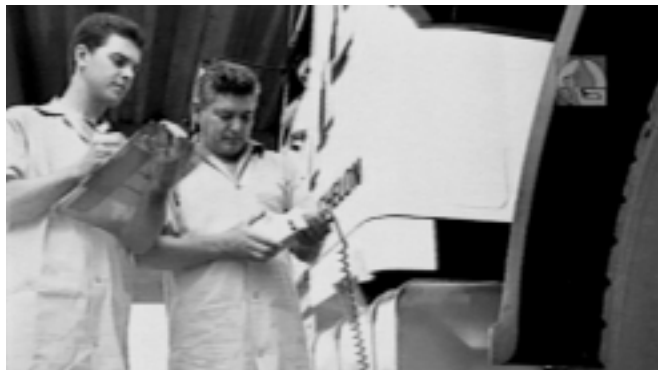
CONPET's transportation programs analyze the opacity of tailpipe emissions to help identify efficiency measures for trucks and buses.
