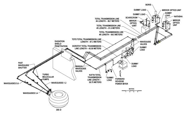
Fig. 1. An overview of the system, including the new addition to the DIII–D experimental facility built to house five gyrotrons.
