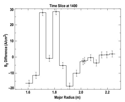
Fig. 4. Although the perturbation in the magnetic field due to rf driven currents is small in the experiments to date, comparison between discharges with and without rf clearly show the presence of these currents through the change in the MSE signals.
