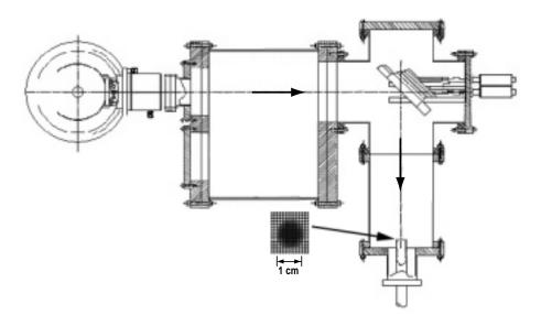
Fig. 3. The single mirror coupling scheme is presented along with the footprint of the beam on thermally sensitive paper at the waveguide input.
