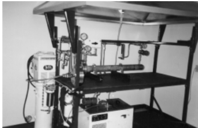
Figure 8. P&ID and photograph of the module testing system used for evaluating the performance of the modules in the laboratory.
