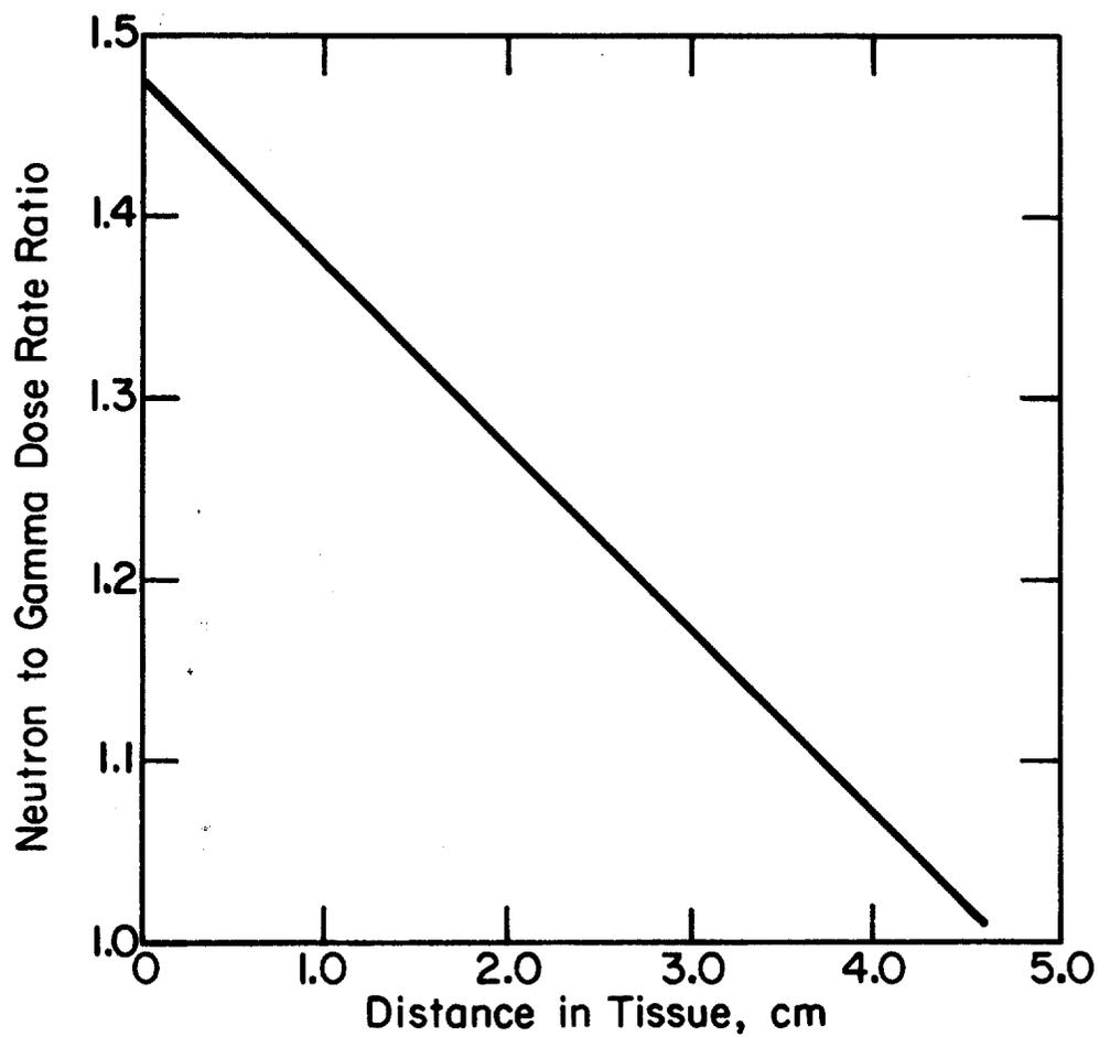
FIG. 3 NEUTRON TO GAMMA-RAY PHYSICAL DOSE RATE RATIO AS A FUNCTION OF TISSUE DEPTH FOR  $^{252}\text{Cf}$
