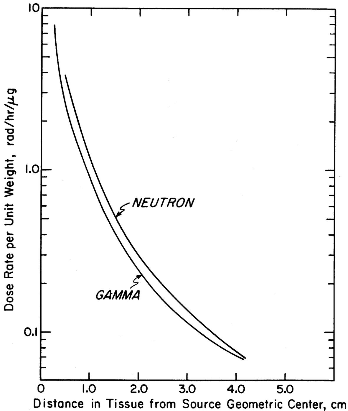
FIG. 2 DISTRIBUTION OF FAST NEUTRON AND GAMMA-RAY DOSE RATE FROM  $^{252}\text{Cf}$  AS A FUNCTION OF TISSUE DEPTH
