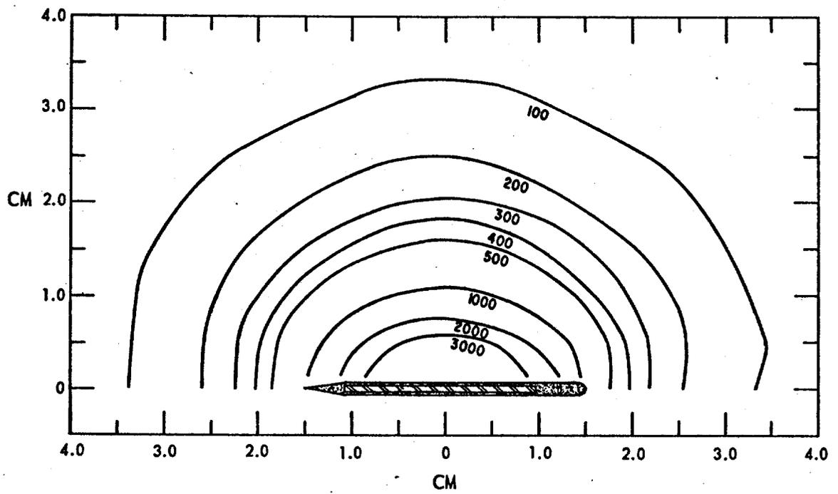
FIG. 5 FAST NEUTRON ISODOSE CHART FOR A  $^{252}\text{Cf}$  NEEDLE IN TISSUE-EQUIVALENT SOLUTION
