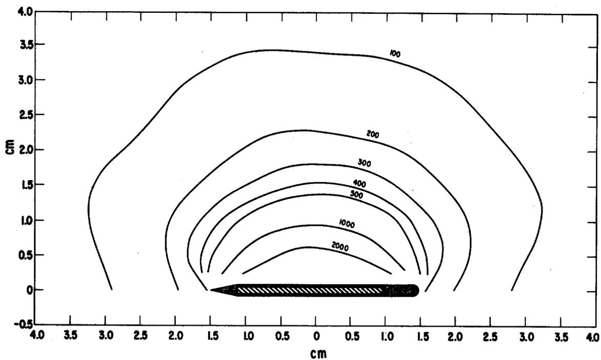
FIG. 6 GAMMA-RAY ISODOSE CHART FOR A  $^{252}\text{Cf}$  NEEDLE
