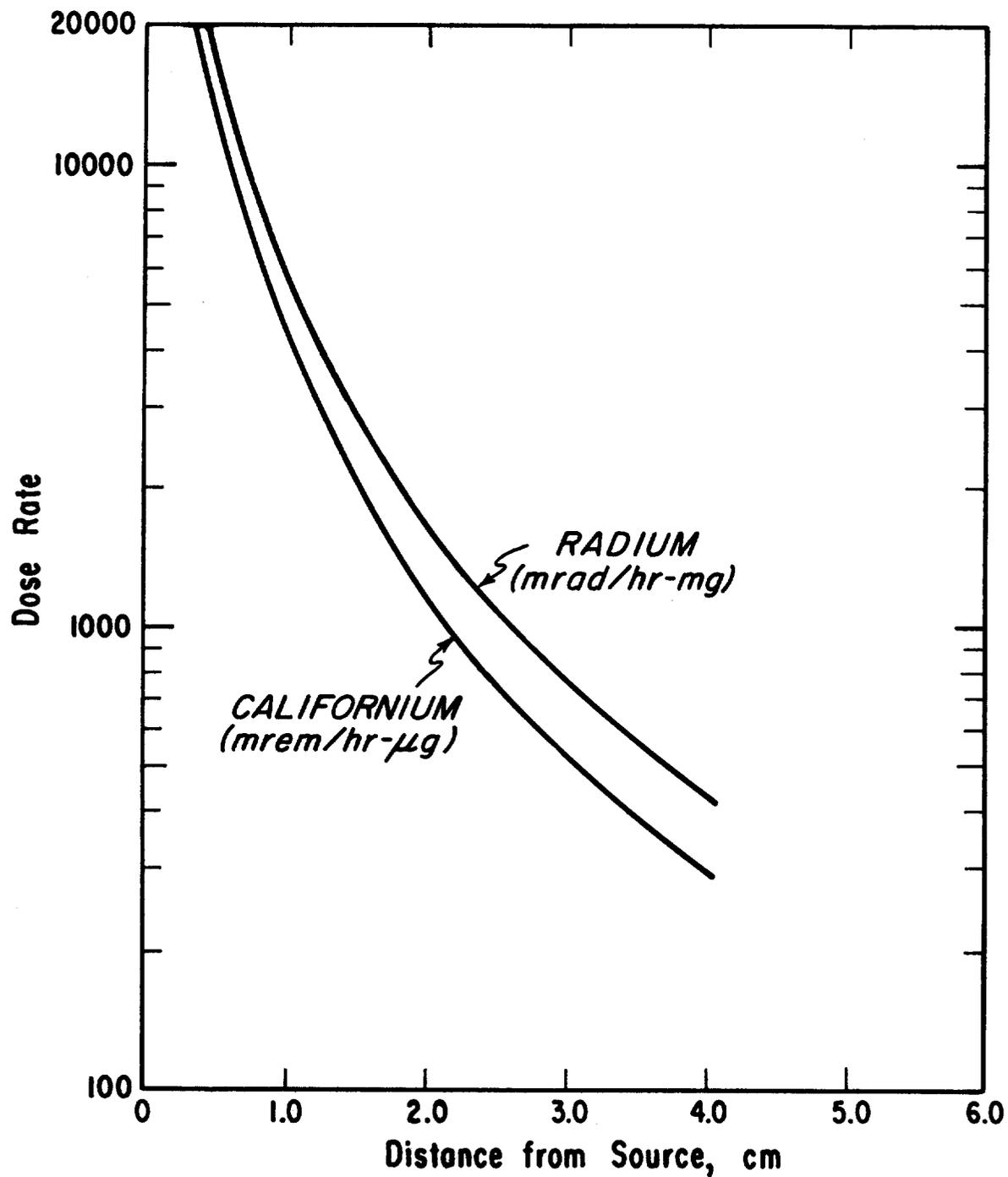
FIG. 4 COMPARISON OF DOSE RATES FROM UNIT WEIGHTS OF  $^{252}\text{Cf}$  AND RADIUM
