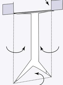
The modified “I”-cut wrap creates three flaps that are wrapped around the window opening
