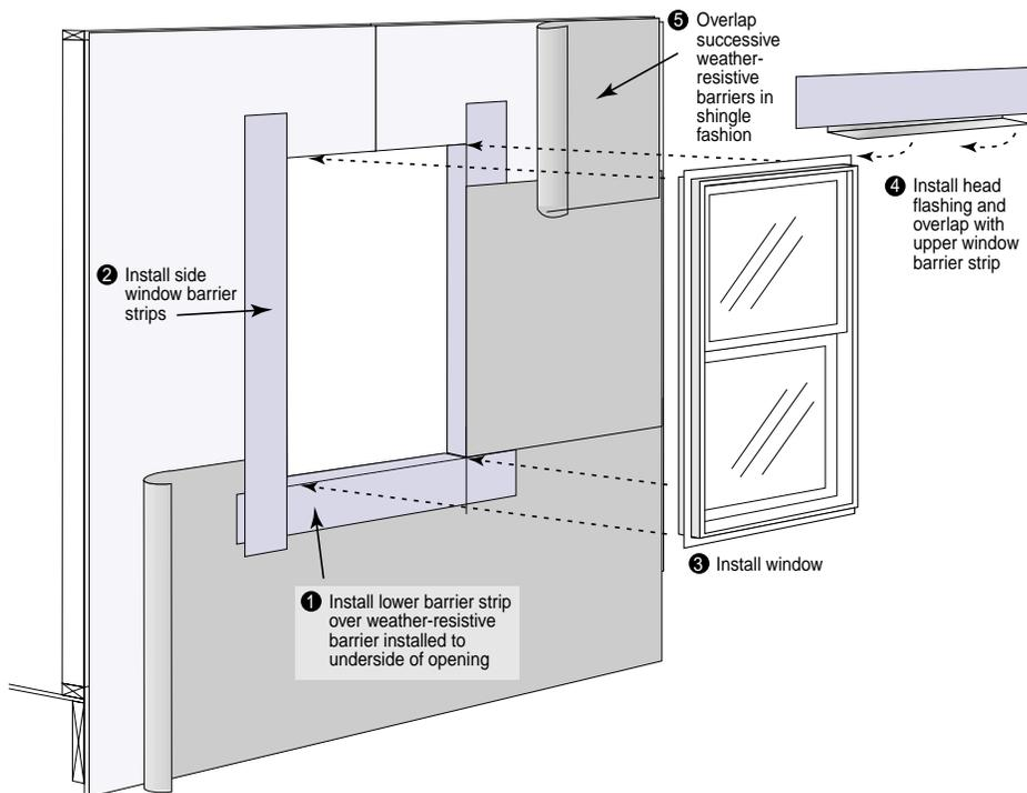
Create slits to slide head flashing and barrier strip underneath housewrap, fasten with nails, then tape the slits in the wrap
